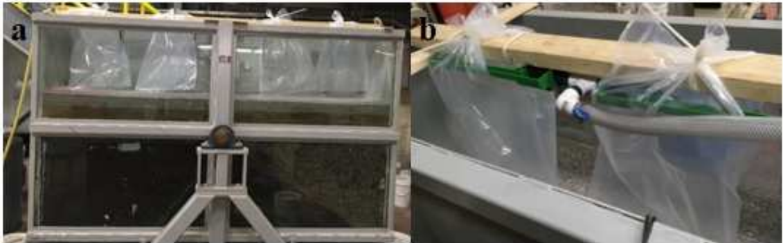
Figure 5.12 Calibration of rainfall simulation system using four plastic bags to collect high pressure water jets from the four oscillating sprinklers
