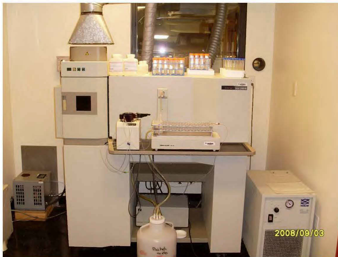
J.9 Photo of the Perkin-Elmer Optima 3100 RL inductively coupled plasma-atomic emission spectroscopy used to determine the chemistry of samples.
