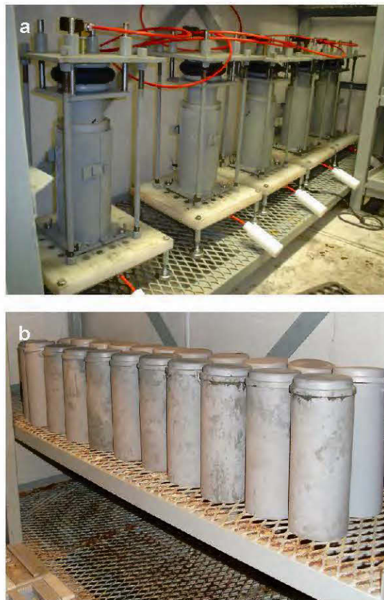
Figure 5.2 Photos of (a) CUAPS-consolidated CPB samples and (b) conventional plastic mould unconsolidated-undrained CPB samples curing in the humidity chamber.
