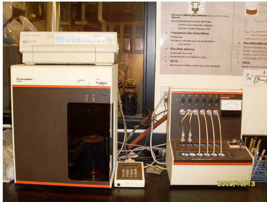
J.7 Photo of the Micromeritics Gemini surface analyzer used to determine the specific surface area of samples.
