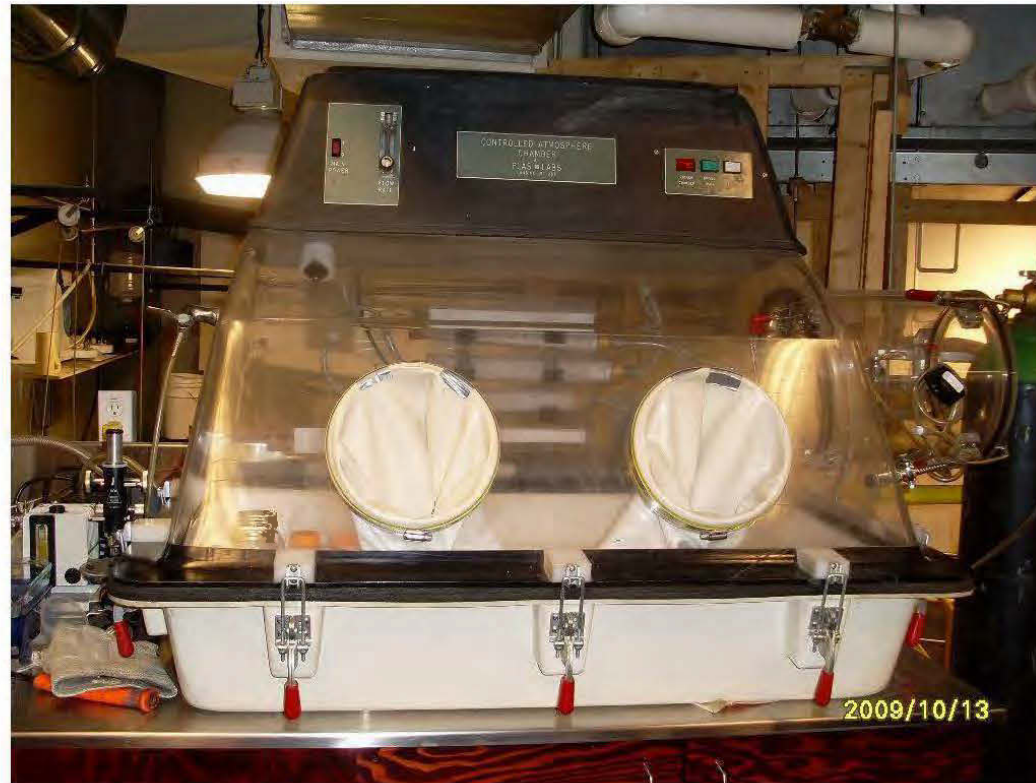
J.16 Photo of the GENEQ Model 855-AC controlled atmosphere chamber for minimizing samples pore alteration due to hydration product destruction and moisture ingress.
