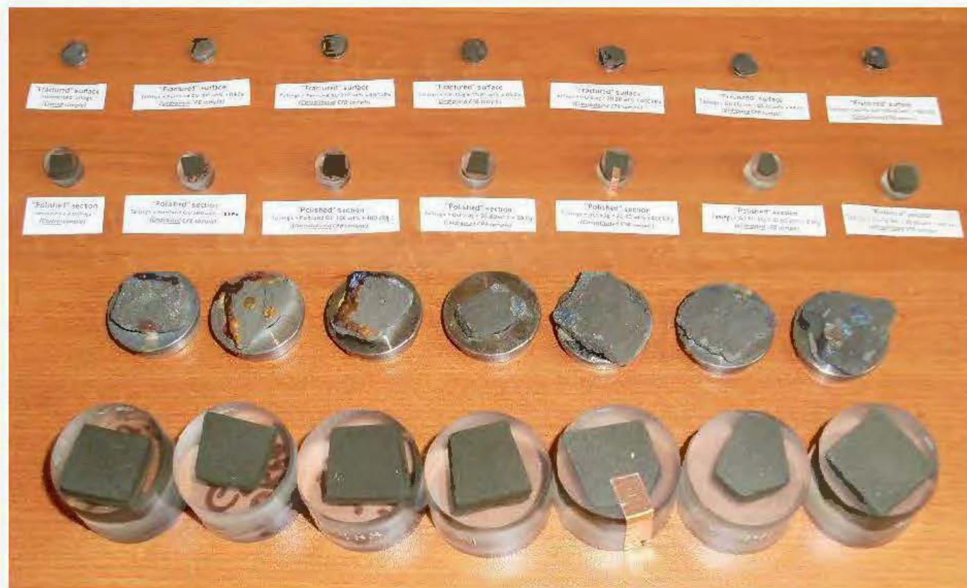
J.20 Photos of polished section and freshly-fractured surface of both uncemented mine tailings and cemented paste backfills containing different binder types such as GU@100 wt%, GU-Slag@20:80 wt% and GU-FA@40:60 wt%.
