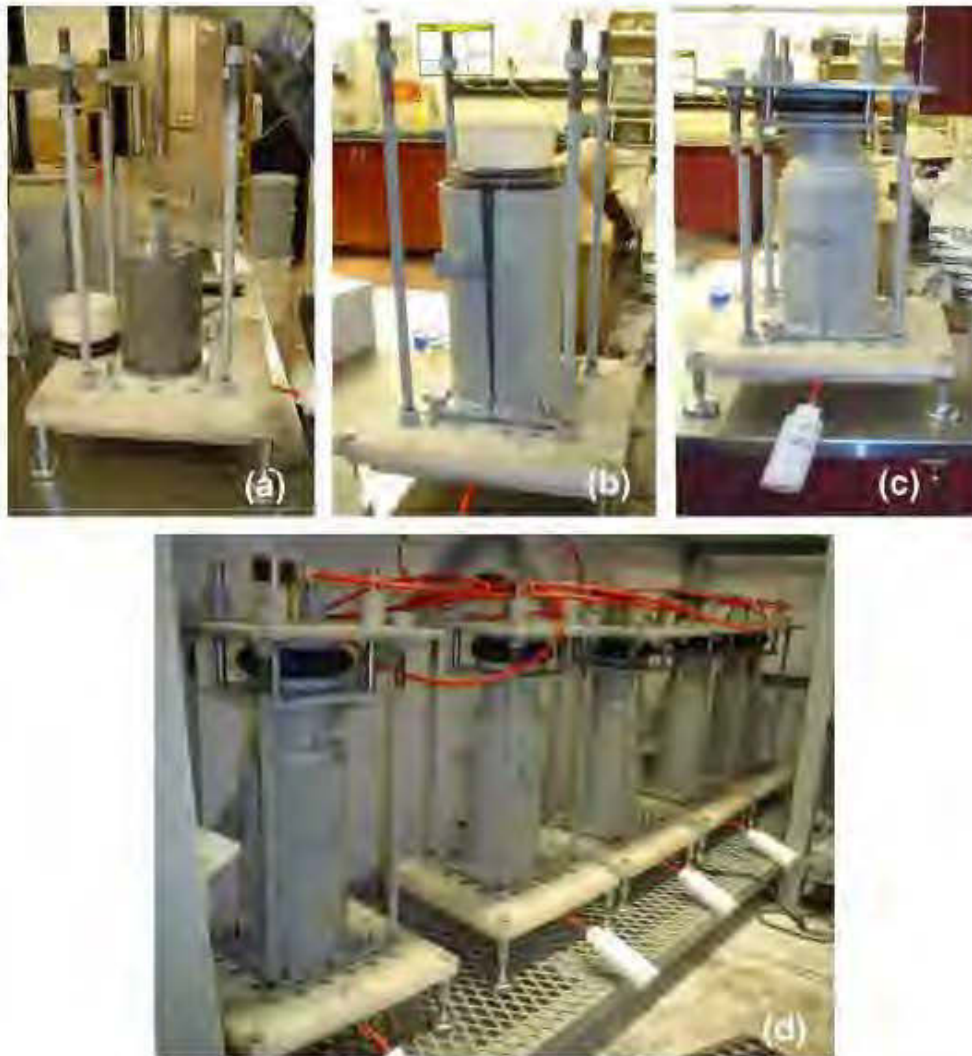
Figure 2.3 Photos illustrating CPB preparation steps: (a) filling Perspex cylinders with CPB material; (b) Perspex cylinder (mould) with supporting cover and PVC loading piston; (c) upper plate equipped with pneumatic pressure application system; and (d) CUAPS cells running tests in a controlled humidity chamber.
