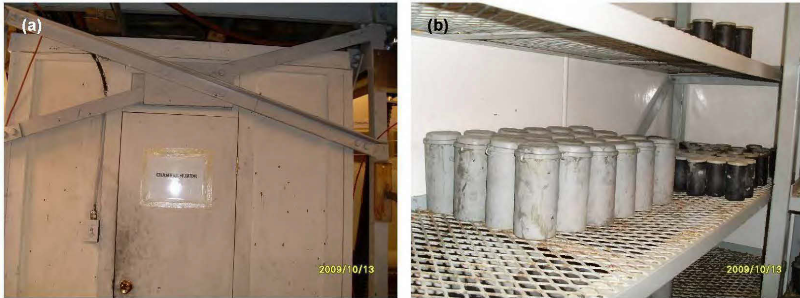
J.11 Photos of (a) an outside view and (b) inside view of the controlled humidity chamber used to cure paste backfill samples.
