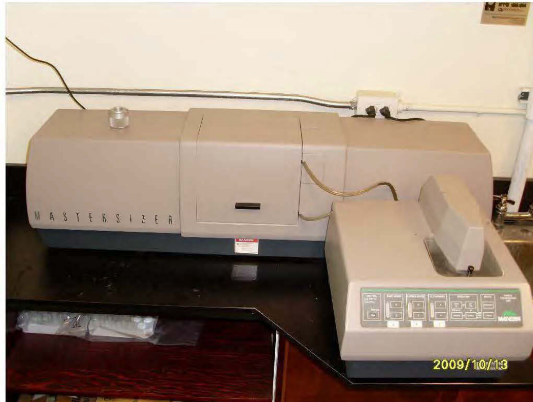
J.5 Photo of the Malvern Mastersizer S200 laser particle size analyzer used to determine the grain size distribution of samples.
