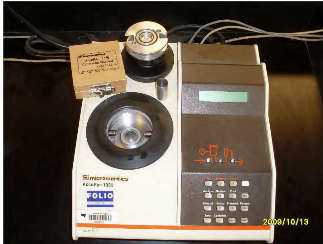
J.6 Photo of the Micromeritics AccuPyc 1330 helium pycnometry system used to determine the specific gravity of samples.
