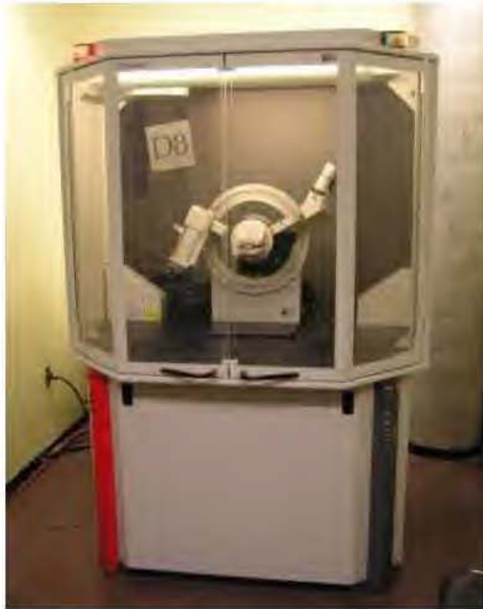
J.8 Photo of the Bruker AXS D8 Advance X-ray diffractometer used to determine the mineralogical composition of samples.
