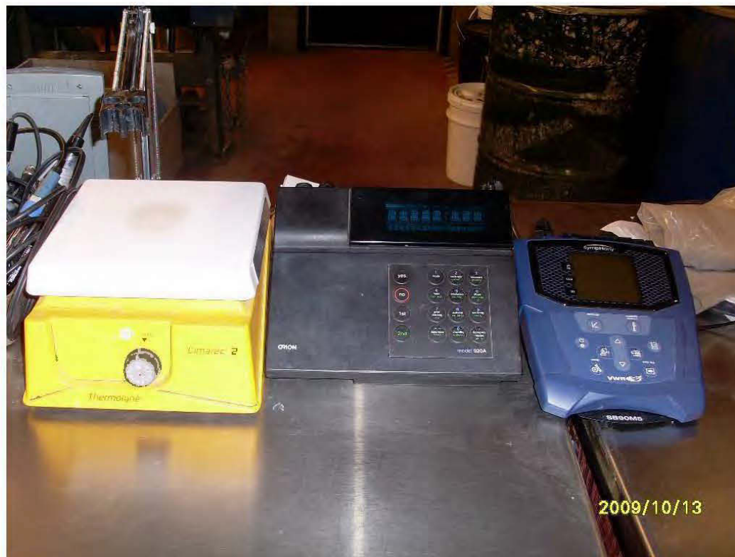
J.10 Photo of the Thermolyne Cimarec 2 Stirrer (left) and the Thermo Fisher Scientific Benchtop Orion Model 920A pH/ISE/mV/ORP/Temperature Meter (right).
