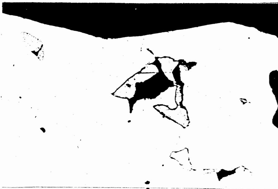
Photomicrograph. x208 - Pyrrhotite (grey) blebs in a recrystallized pyrite grain. The pyrrhotite outlines are in part controlled by the pyrite grain boundaries.
