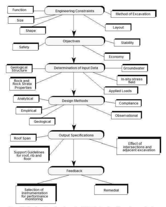
Figure 3: The flow chart showing a simplified design chart for underground mine design
