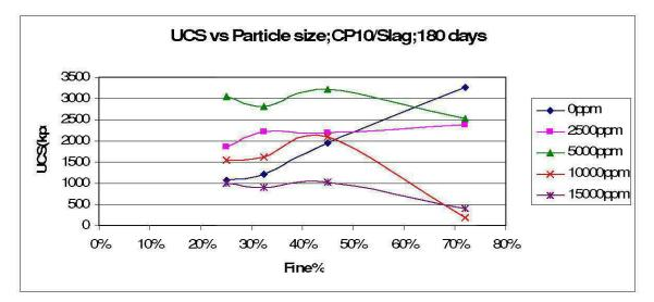
Figure 34: UCS vs Particle size; CP10: Slag; 180 days
