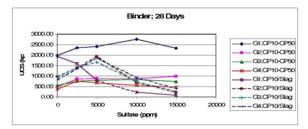
Figure 21: UCS according to the content sulfates for the CP10-CP50 and CP10-Slag (28 days of cure)
