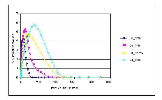
Figure 8: Histogram of Particle size distributions of the silica powder
