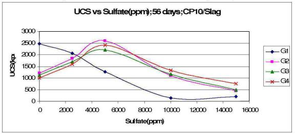
Figure 42: UCS vs Sulfate content; CP10: Slag; 56 days
