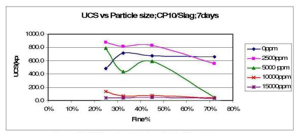
Figure 30: UCS vs Particle size; CP10: Slag; 7 days
