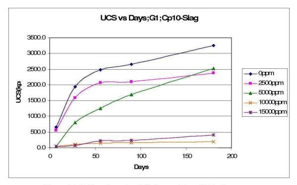
Figure 16: UCS vs Days for 72% fine particles; CP10: Slag
