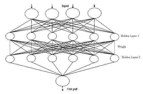
Figure 5: Structure of multi-layered type artificial neural network
