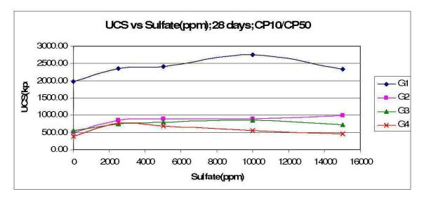
Figure 36: UCS vs Sulfate content; CP10:CP50; 28 days
