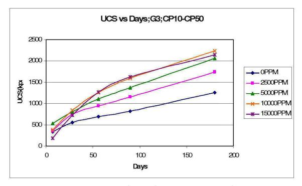
Figure 14: UCS vs Days for 32% fine particles; CP10:CP50
