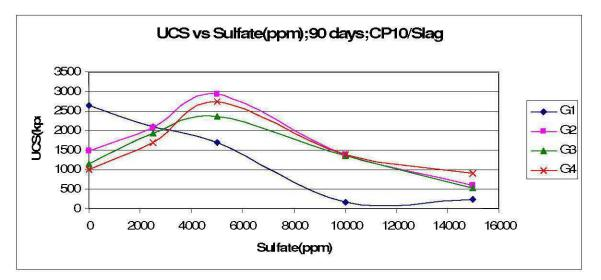
Figure 43: UCS vs Sulfate content; CP10: Slag; 90 days
