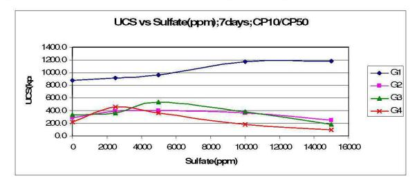
Figure 35: UCS vs Sulfate content; CP10:CP50; 7days
