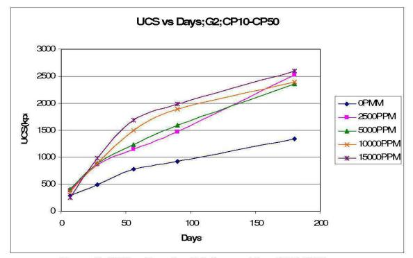
Figure 13: UCS vs Days for 45% fine particles; CP10:CP50
