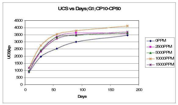
Figure 12: UCS vs Days for 72% fine particles; CP10:CP50
