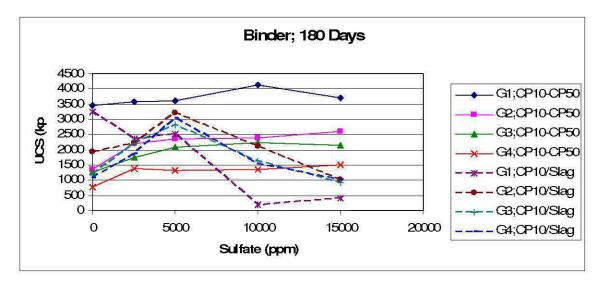
Figure 24: UCS according to the content sulfates for the CP10-CP50 and CP10-Slag (180 days of cure)
