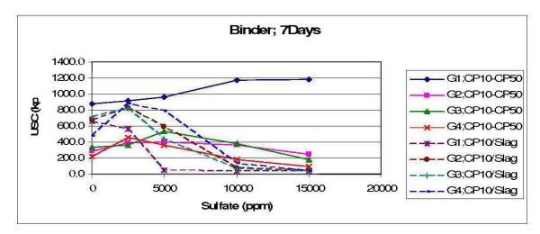
Figure 20: UCS according to the content sulfates for the CP10-CP50 and CP10-Slag (7 days of cure)
