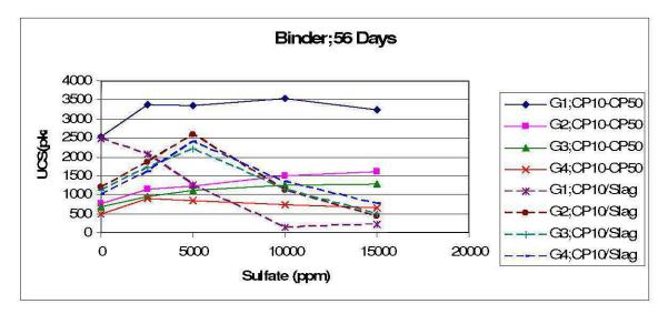
Figure 22: UCS according to the content sulfates for the CP10-CP50 and CP10-Slag (56 days of cure)
