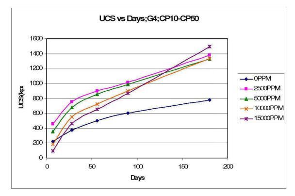
Figure 15: UCS vs Days for 25% fine particles; CP10:CP50
