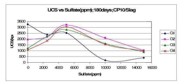
Figure 44: UCS vs Sulfate content; CP10: Slag; 180 days
