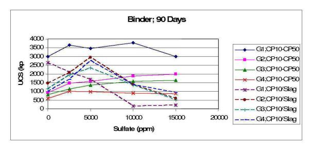
Figure 23: UCS according to the content sulfates for the CP10-CP50 and CP10-Slag (56 days of cure)
