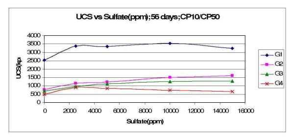
Figure 37: UCS vs Sulfate content; CP10:CP50; 56 days
