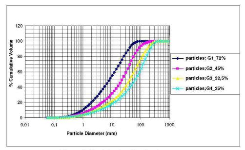
Figure 7: Particle size distribution curves
