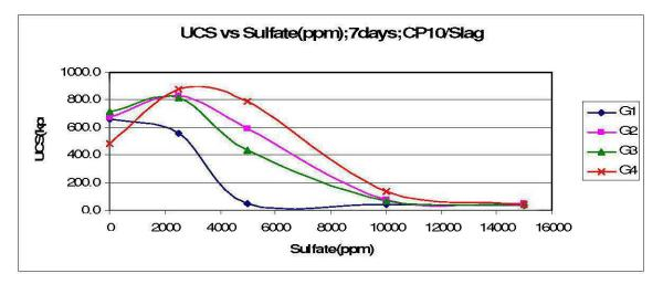
Figure 40: UCS vs Sulfate content; CP10: Slag; 7 days
