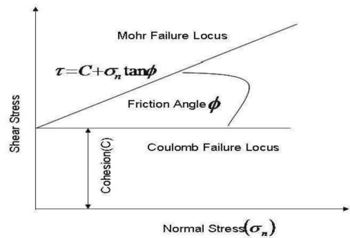
Figure 2: Mohr Failure Locus
