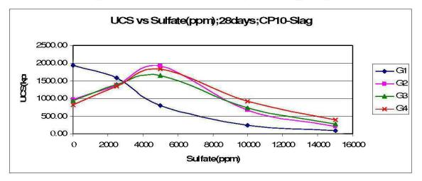
Figure 41: UCS vs Sulfate content; CP10: Slag; 28 days
