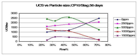
Figure 32: UCS vs Particle size; CP10: Slag; 56 days
