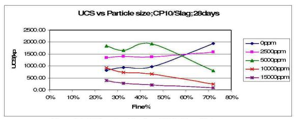
Figure 31: UCS vs Particle size; CP10: Slag; 28 days
