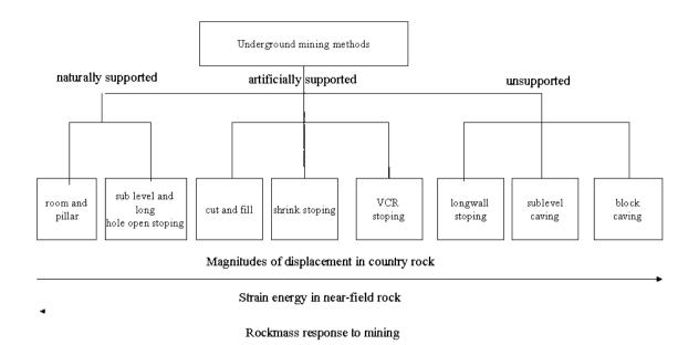
Figure1: Diagram showing a breakdown of mining methods according to the mine regional support system used, Brady and Brown (2004)
