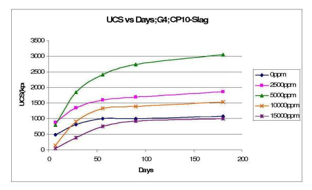
Figure 19: UCS vs Days for 25% fine particles: CP10: Slag
