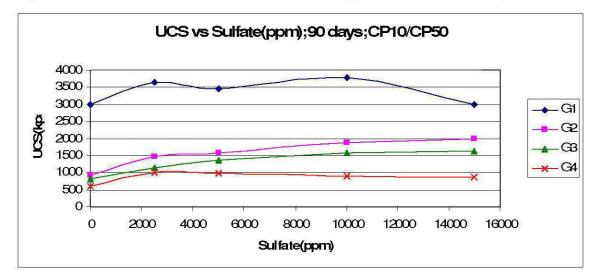
Figure 38: UCS vs Sulfate content; CP10:CP50; 90 days
