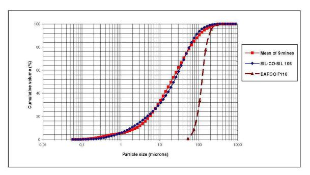
Figure 6: Particle size distribution of the silica products
