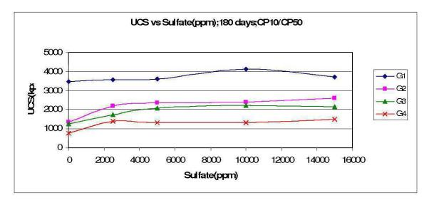
Figure 39: UCS vs Sulfate content; CP10:CP50; 180 days
