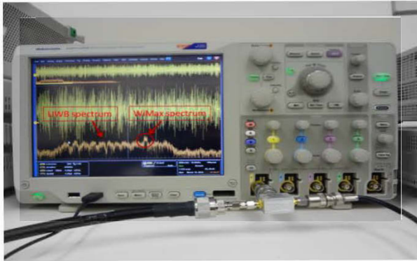
UWB received spectrum in the presence of WiMAX with separation distance of 5m.
