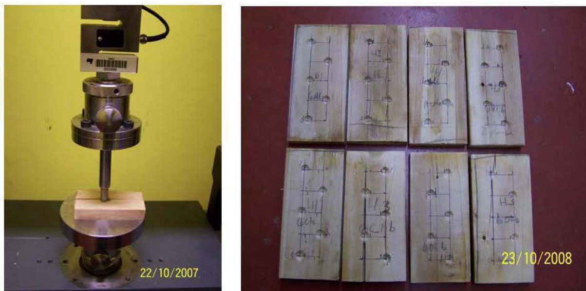
Figure 4.16: Splits in the samples during the Janka hardness test.
