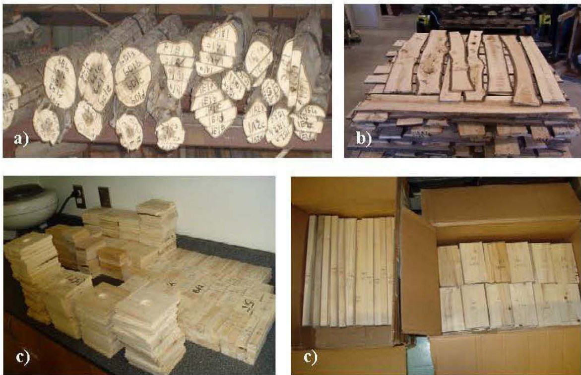
Figure 3.2: a) Hybrid poplar boards after sawing; b) Hybrid poplar boards after drying; c) Final specimens for different tests.
