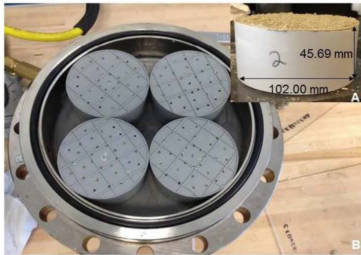
Figure 3.1: Molded rock-bentonite mixture (A) and pressure plate apparatus sample set-up (B).
