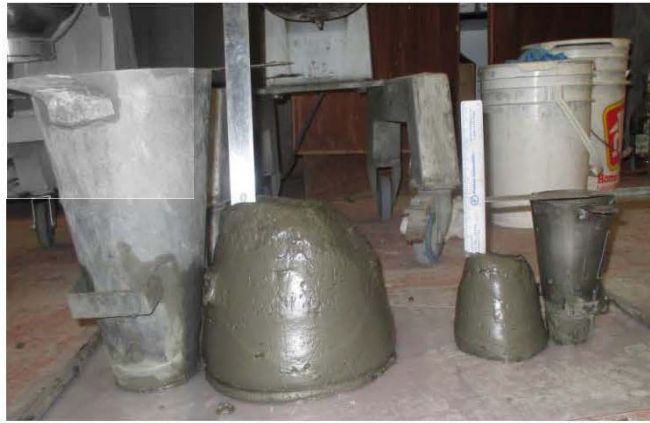
Fig. 3.2 Example of a standard cone (left) and a mini-cone (right) for slump tests on CPB incorporating HRWR polymers.
