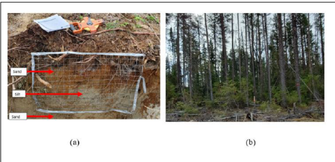
Figure C.8.4 (a) The substrate profile of the selected site for the NA of a CCBE, composed of sand layers above and below a silt layer; (b) The selected site for the NA of a CCBE is colonised by mature jack pine vegetation
