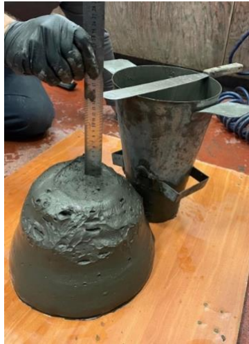
Figure 4 Slump measurement using the standard Abrams cone method
