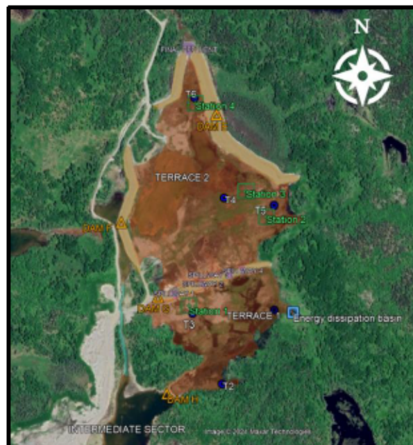
Figure 6.1: Northern part of the Aldermac site reclaimed using the elevated water table technique combined with a monolayer cover of sand and gravel (aerial photo from Google Earth).
