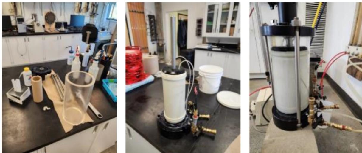
Figure 3.16 The process of preparation and testing of samples in saturated hydraulic conductivity analysis
