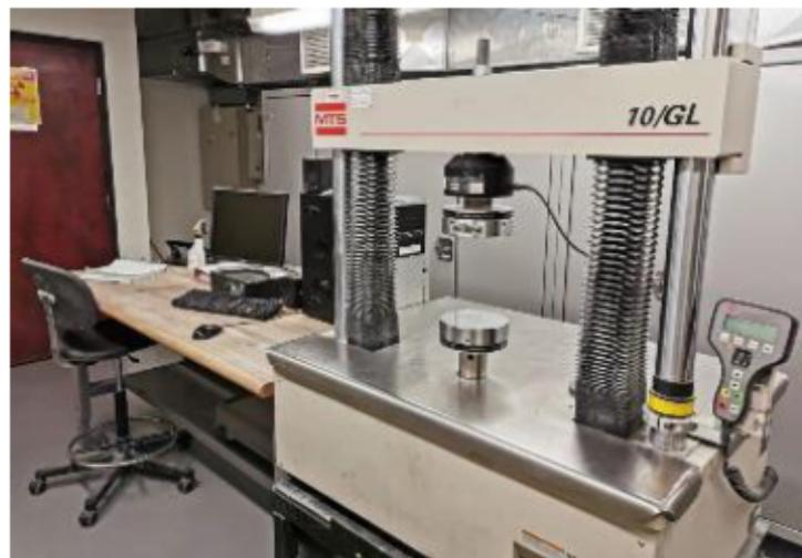
Figure 3.15 A view of the UCS test apparatus and data acquisition system
