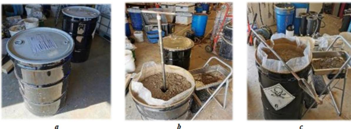
Figure 3.10 A view of a) two barrels of tailings of the Giant Mine, b) sampling from the whole height of each barrel, c) a view of the hand auger and the collected sample
