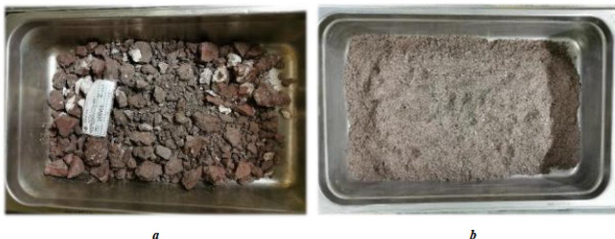
Figure 3.5 Dust sample B233-P9, a) before, b) after grinding with roller mill
