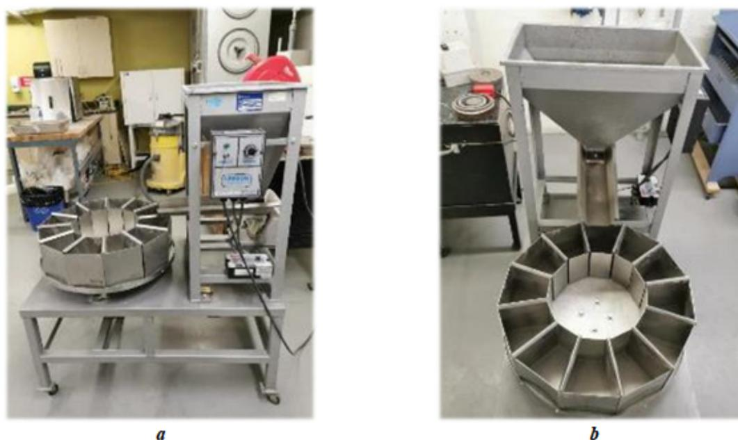
Figure 3.7 Rotary sample splitter, a) side view that shows the controller, b) front view
