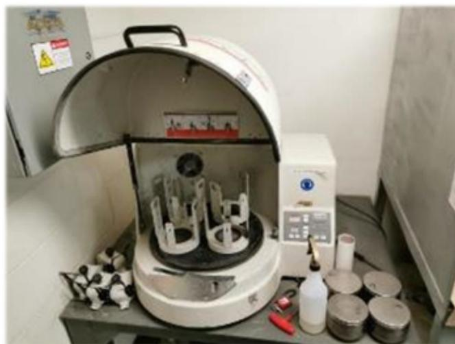
Figure 3.3 The planetary ball mill with 4 cylinders
