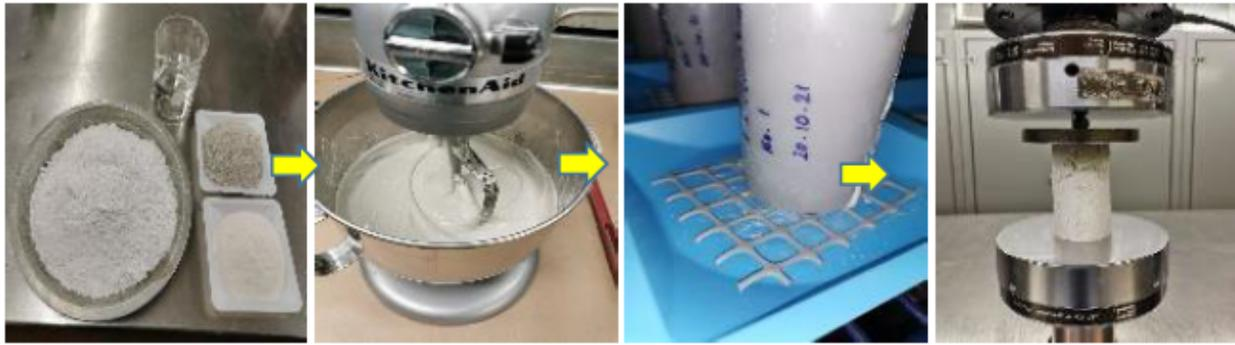
Figure B.1 Process of preparation, mixing, curing, and testing of the cemented paste backfill samples
