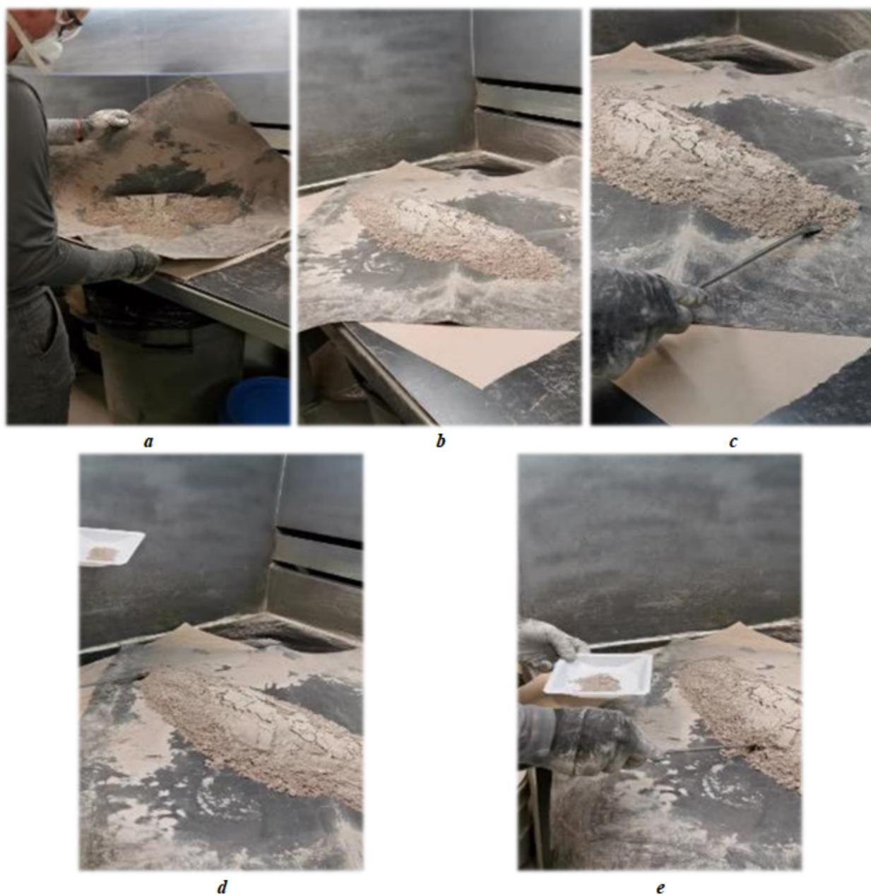
Figure 3.6 Different steps of homogenization, preparation, and sampling of ATRW dusts, a) rolling at different directions, b) the final row of material, c) sampling from the right end, d) sampling from the left end, e) sampling from the center of the mass
