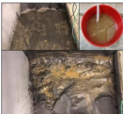
Figure 4.28. Visible superficial erosion for FCL with 10° slope.
