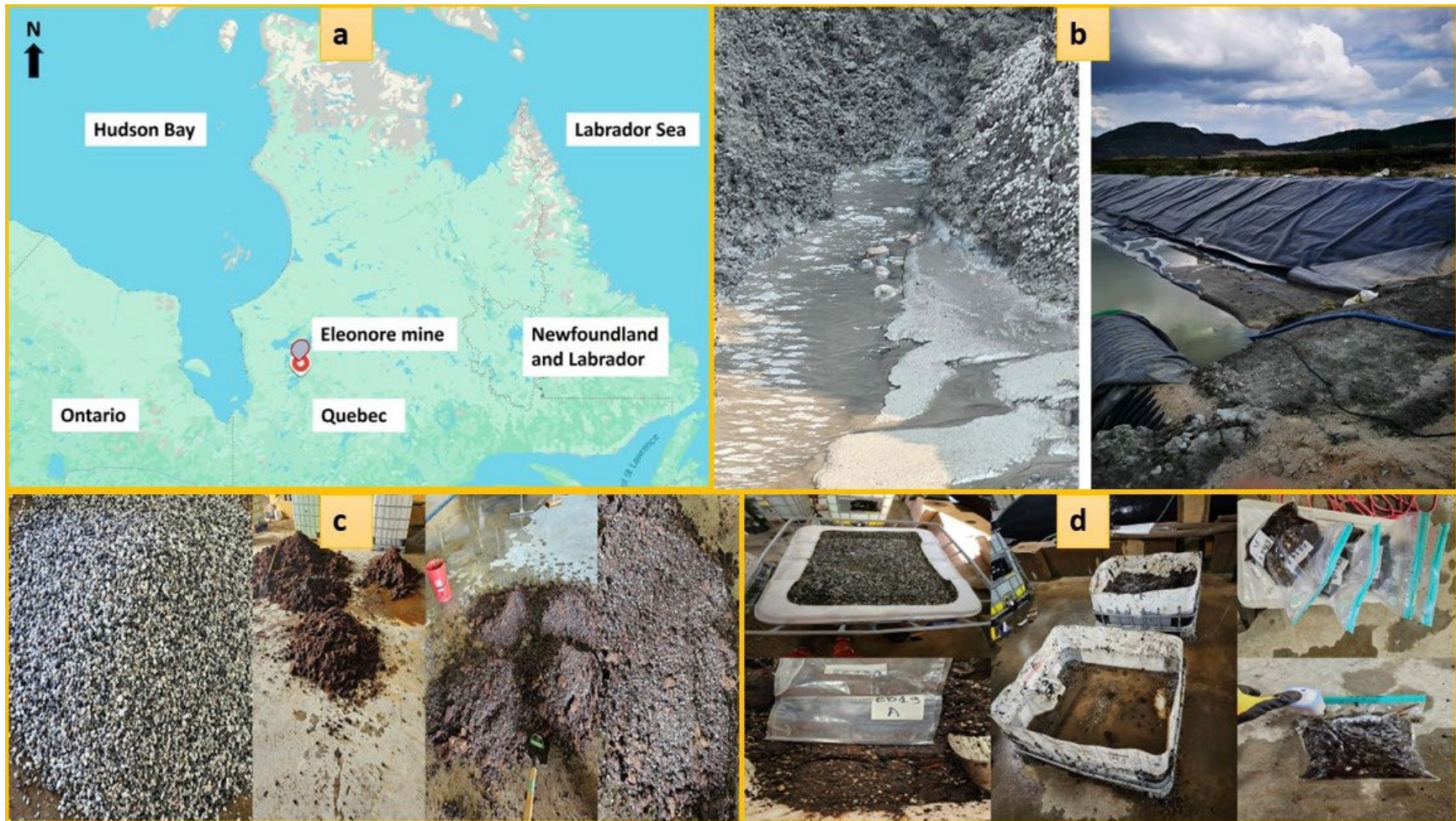
Figure B1. Field experimental work: a) Site location (adapted from https://www.google.ca/maps ), b) On-site sampling of As-CND, c) Preparation of the reactive mixture, d) Sampling of post-treatment residues of field-pilot biofilters
