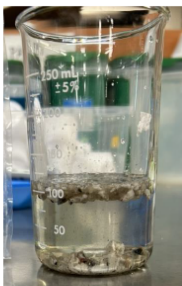
Figure 3.6 Completed HLS test showing a clear separation of particles into sink and float fractions.
