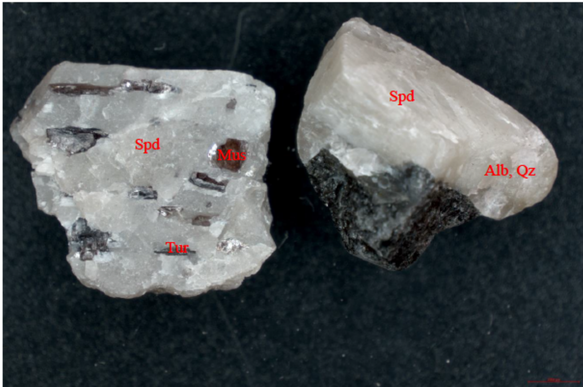
Figure 4.8 Optical microscopy image on the mixed spodumene sample (+6.3mm, 2.85g/cm 3 ). Spodumene (spd), muscovite (Mus), tourmaline (Tur), albite (Alb), and quartz (Qz) are marked in the image.
