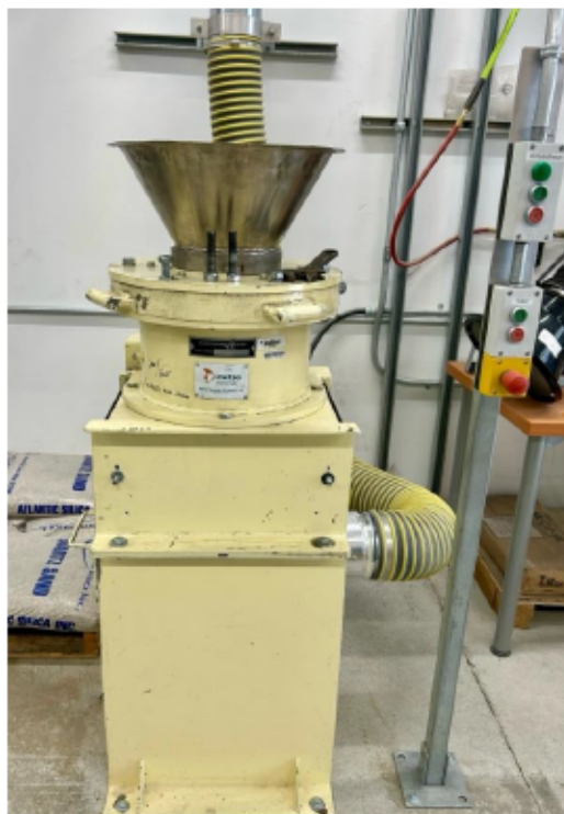
Figure 3.2 Metso Minerals Marcy cone crusher.
