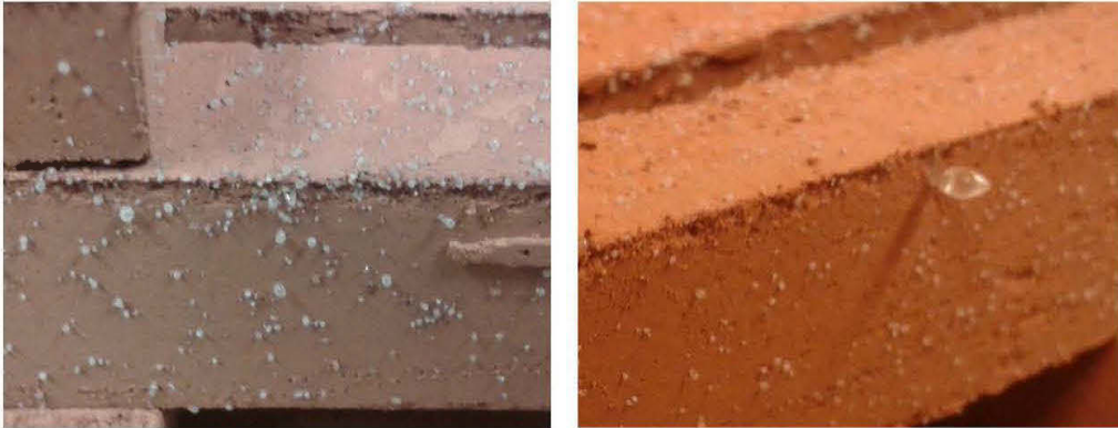
Figure 6.6 Entrapped gas pockets at the surface of bricks containing 15% of glass wastes (GW).
