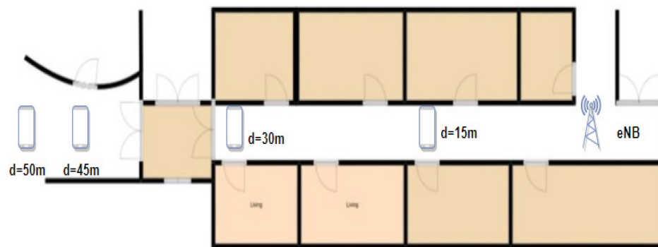
Figure 44: Map of the indoor corridor with the LTE measurement setup.
