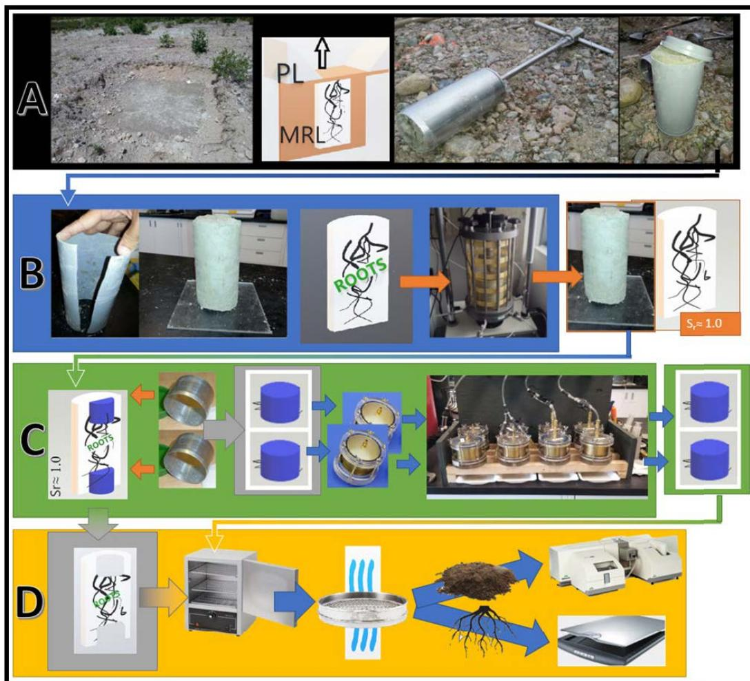
Figure 4.3 (A) Diagram of the manipulations carried out on each sample from field sampling, (B) Preparation and execution of the flexible wall permeameter test, (C) Transfer from the triaxial cell to the Tempe cells, and (D) Drying and separation of soil and roots for grain-size distribution and root parameters analysis
