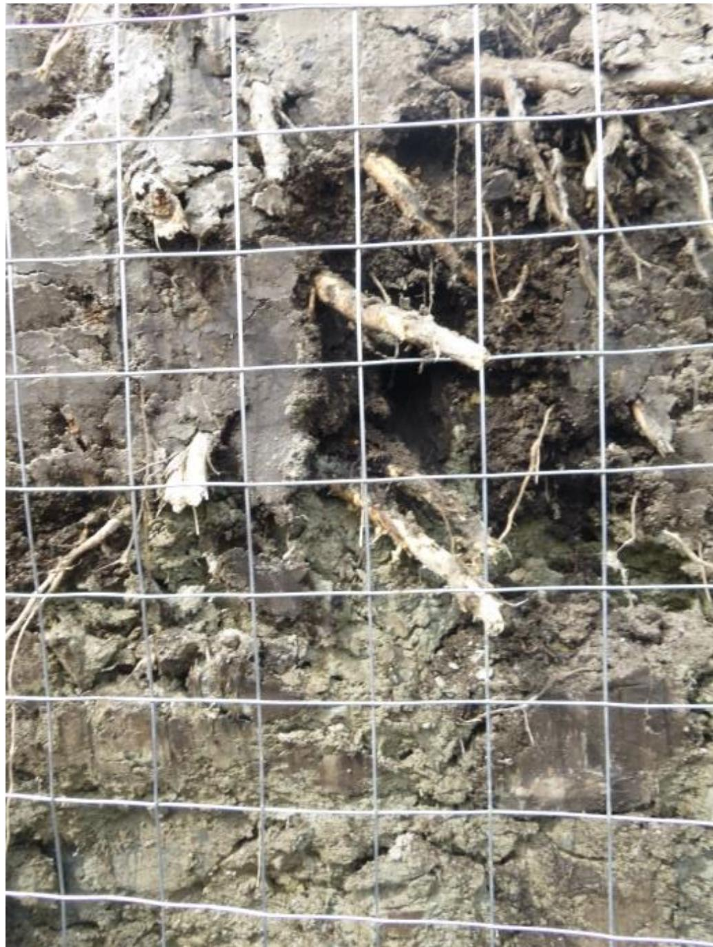
Figure 5.3 Root count grid applied to the vertical walls of the trenches
