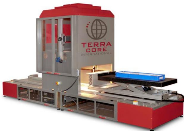
**Figure 2-10: Appareil ROCK (2/3 sensor) de la compagnie Terracore (Terracore, 2021)**
