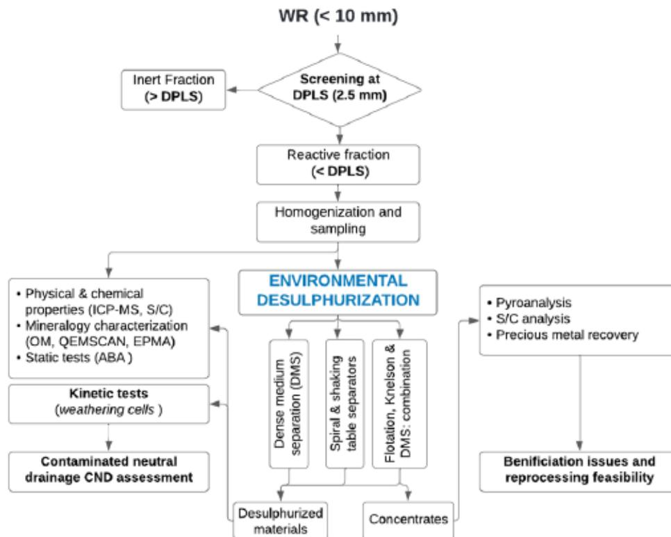
Figure 7.1 Methodology followed for WR characterisation and desulphurization to assess contaminated mine drainage generation and the recovery of precious metals.
