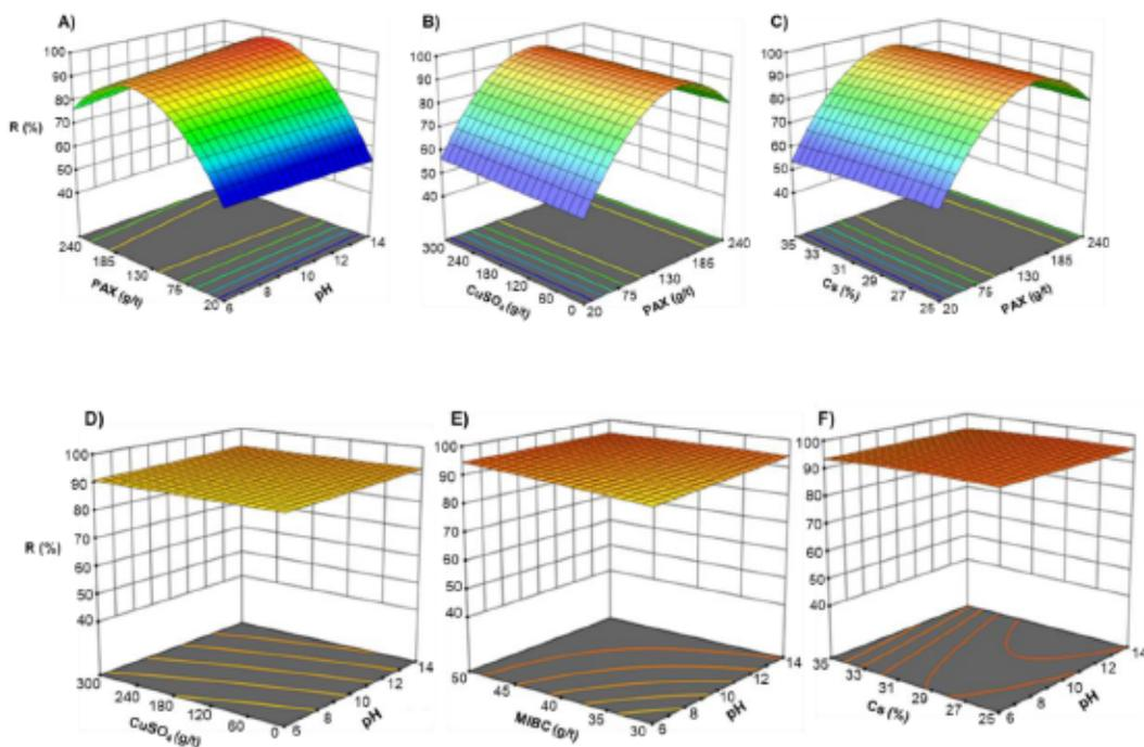
Figure 5.8 The three-dimensional quadratic response surfaces for total sulfur recovery with A) PAX vs pH with  $\text{CuSO}_4=200$  (g/t), and MIBC=40 (g/t); B)  $\text{CuSO}_4$  vs PAX for pH=10 & MIBC=50 (g/t); C) Cs vs PAX for pH=10,  $\text{CuSO}_4=210$  (g/t), and MIBC=40(g/t); D)  $\text{CuSO}_4$  vs pH for PAX=120 (g/t) and MIBC=40 (g/t); E) MIBC vs pH for PAX=130 (g/t) and  $\text{CuSO}_4=300$  (g/t); F) Cs vs pH for PAX=130 (g/t),  $\text{CuSO}_4=300$  (g/t), and MIBC=50 (g/t).
