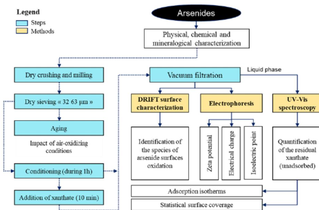
Figure 4.1 Methodology illustrating the experimental work followed to investigate the surface physicochemistry of the studied arsenide minerals.
