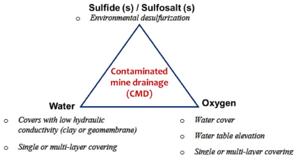
Figure 2.1 Trigger components of CMD generation and some control methods
