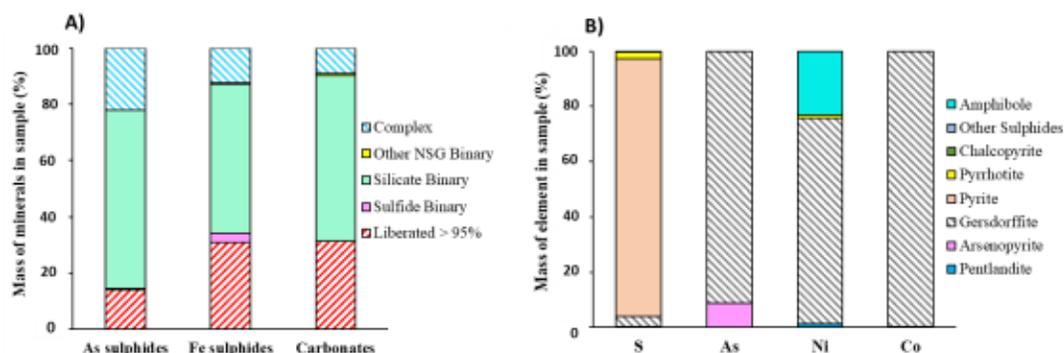
Figure 7.6 A) Mineralogical associations and B) sulphur, arsenic, nickel, and cobalt deportments for the feed sample.
