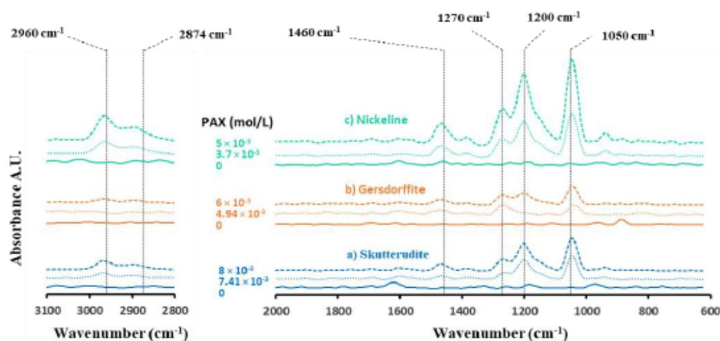
Figure 4.8 Diffuse infrared spectra from 2,000 to 600  $\text{cm}^{-1}$  and 3,100 to 2,800  $\text{cm}^{-1}$  for the studied arsenides under optimal adsorption conditions and with various xanthate concentrations: a) skutterudite, b) gersdorffite, and c) nickeline.
