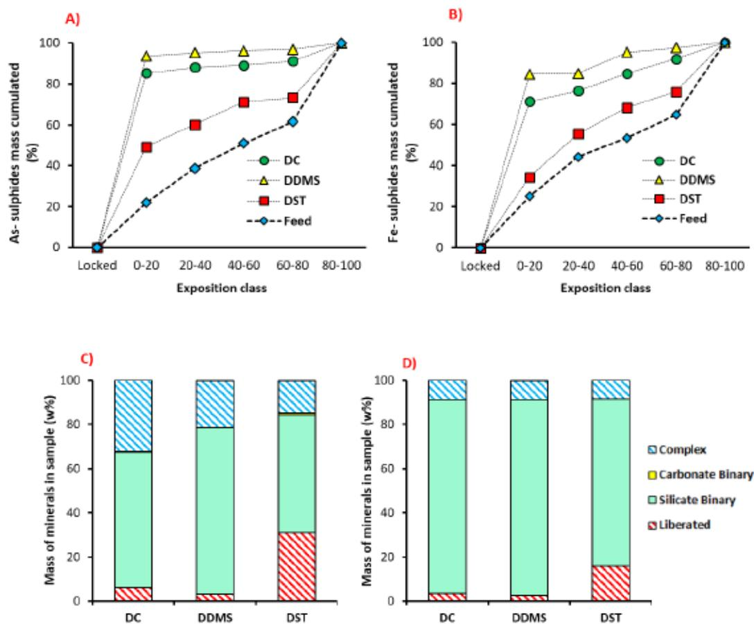
Figure 7.7 Mineral liberation degree of A) As-sulphides, B) Fe-sulphides, and mineralogical associations of C) As-sulphides and D) Fe-sulphides for the desulphurized materials.
