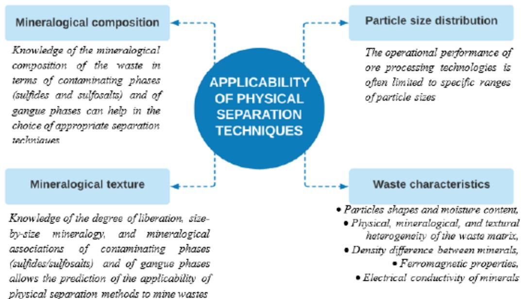
Figure 2.9 The different parameters used for defining the applicability of physical separation techniques to environmental desulfurization of mine wastes.
