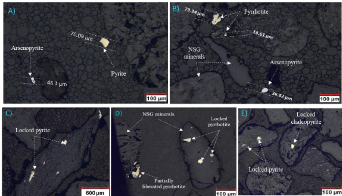
Figure 7.13 Optical microscopy of the polished section of the desulphurized material using A, B) spiral/shaking table approach and C, D, E) combination approach.
