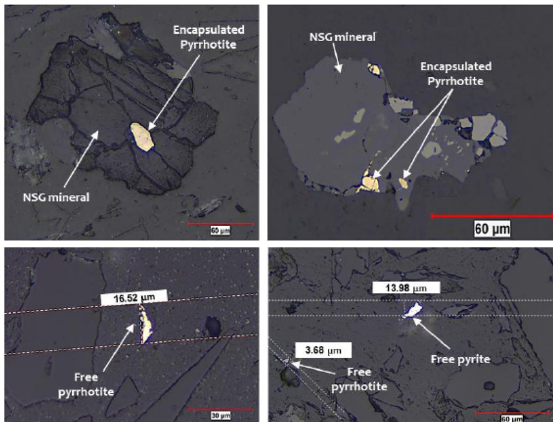
Figure 5.11 Optical microscopy of the polished section of desulfurized tailings.
