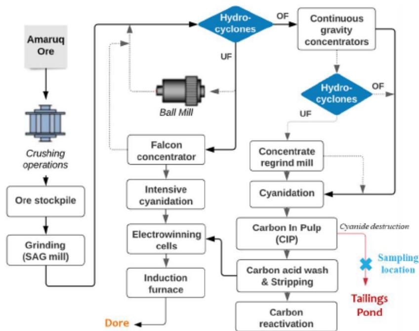
Figure 5.1 Simplified Amaruq processing flowsheet and sampling location.
