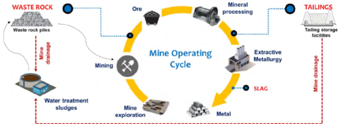
Figure 2.2 The operating cycle of a mine and the main typologies of mine wastes.
