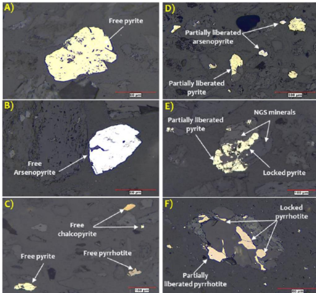
Figure. 5.4 Optical microscopy (reflected light mode) photomicrographs of the studied tailings highlighting the textures and mineralogical associations of sulfides and gangue minerals.
