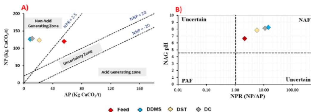
Figure 7.8 Classification of the feed sample and the desulphurized materials in terms of A) acid-base accounting tests and B) NPR versus NAG pH (NAF: non-acid forming; PAF: potentially acid-forming).
