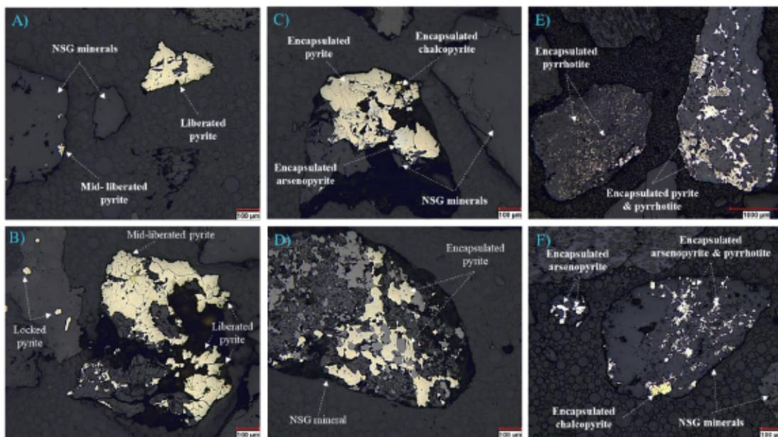
Figure 7.4 Optical microscopy (reflected light mode) photomicrographs of the studied material showing textures and mineralogical associations of sulphides. A, B) Liberated and mid-liberated sulphides, C, D, E, and F) encapsulated sulphides.
