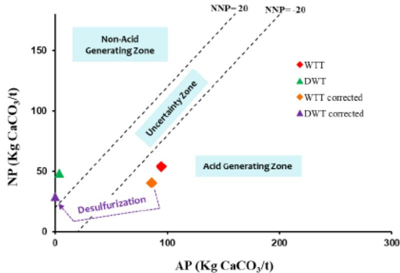
Figure 5.12 WTT and DWT classification in terms of absolute AP and NP and available AP and NP after correcting for the sulfide and carbonate liberation degrees.
