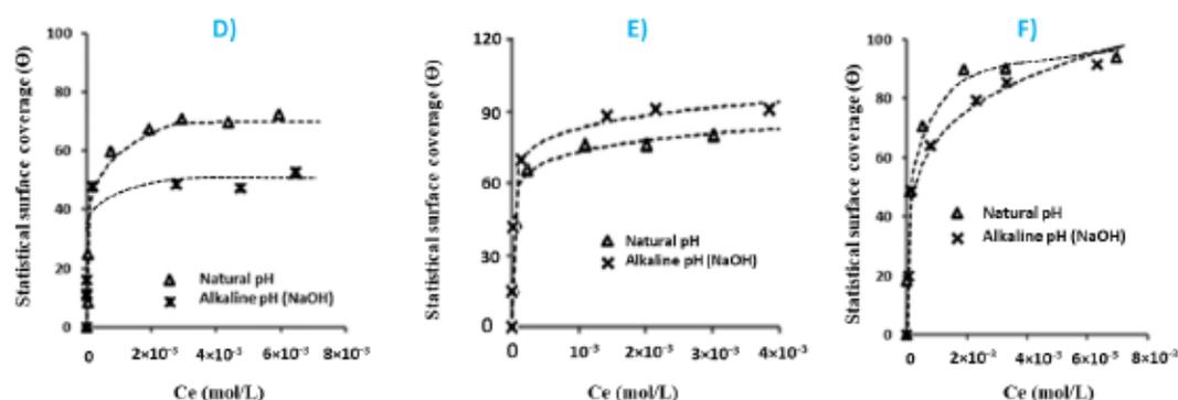
Fig. 4.7 Adsorption isotherms for the xanthate collector on different mineral surfaces after activation with  $\text{CuSO}_4$  and under natural and alkaline conditions: D) skutterudite, E) gersdorffite, and F) nickeline.
