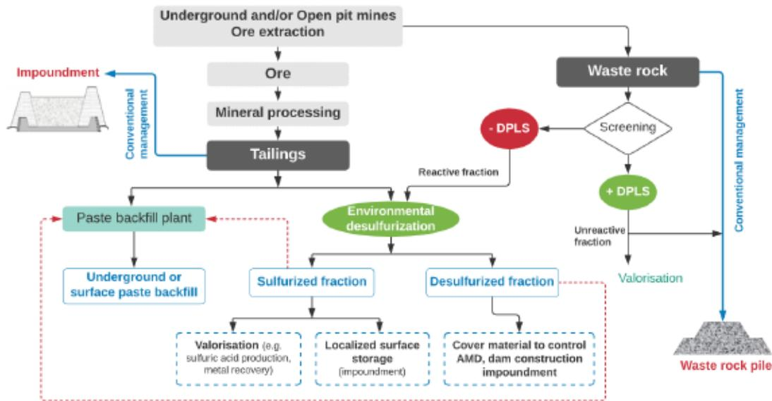
Figure 2.6 Approaches to reach an integrated mine waste management
