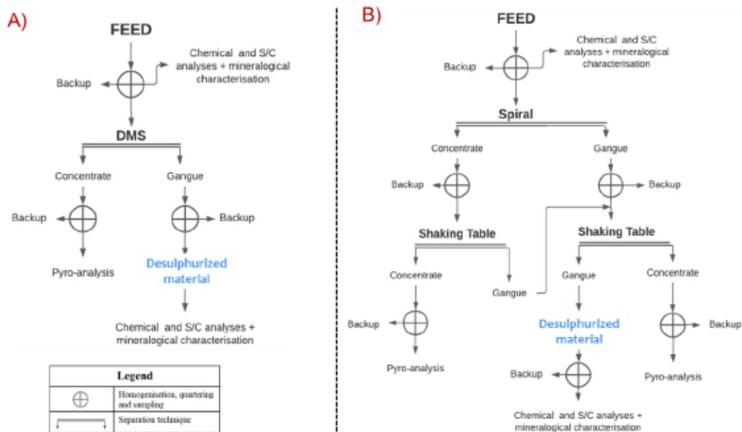
Figure 7.2 A process flow chart of the different decontamination techniques used: A) DMS approach, B) spiral/shaking table approach, and C) combination gravity and flotation approach.
