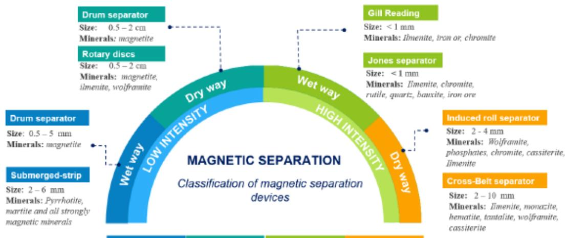
Figure 2.8 Application and particle size limits of magnetic separators
