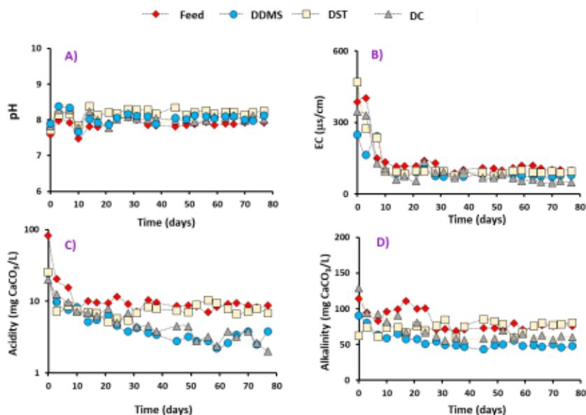
Figure 7.9 A) pH, B) electrical conductivity, C) acidity, and D) alkalinity evolution within the leachates from the feed and desulphurized materials.
