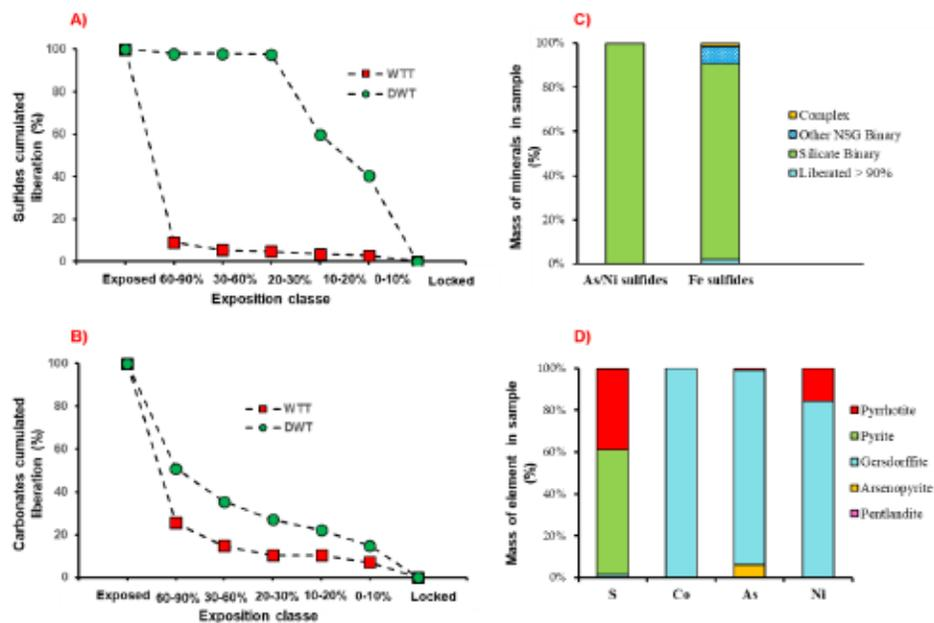
Figure 5.10 Mineral liberation of (A) sulfide and (B) carbonate minerals within the WTT and DWT samples. C) Mineralogical associations of sulfide minerals within the DWT. D) Sulfur, cobalt, arsenic, and nickel departments for DWT.
