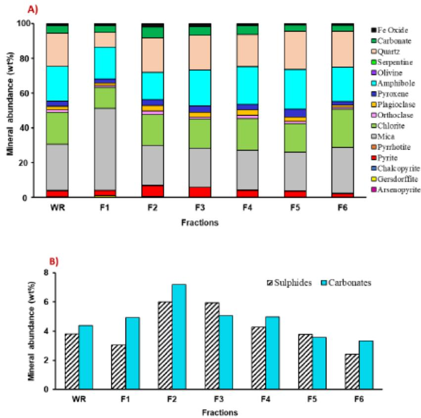
Figure 6.4 A) Mineralogical compositions of the studied WR (total sample) and its corresponding grain-size fractions using QEMSCAN® analysis, and B) carbonates and sulphides distributions within the studied WR and grain-size fractions.
