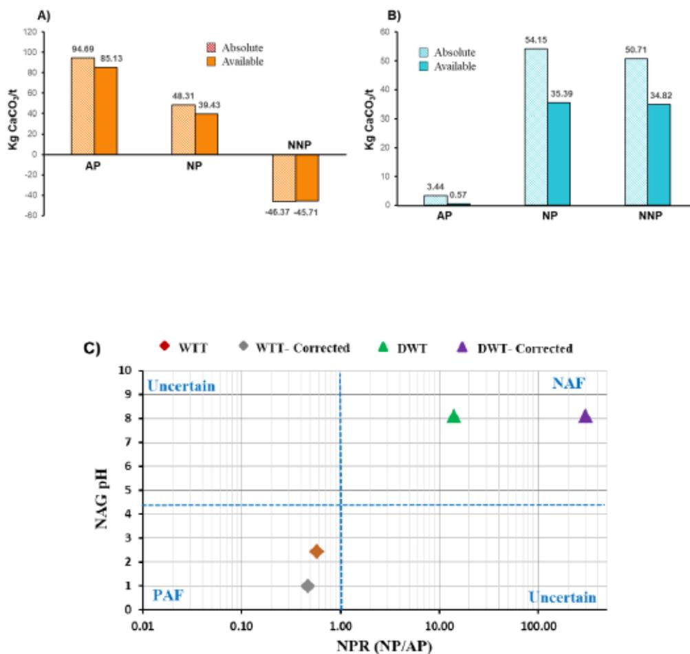
**Figure S1.2** Absolute and available (after correction with liberation degree) AP, NP, and NNP for A) WTT and B) DWT. C) Results of acid generation potential from ABA and NAG tests.
