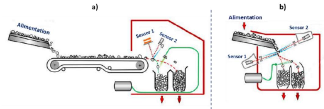
Figure 3S. Automated sorting systems a) belt, b) free fall. Adapted from Wills,
