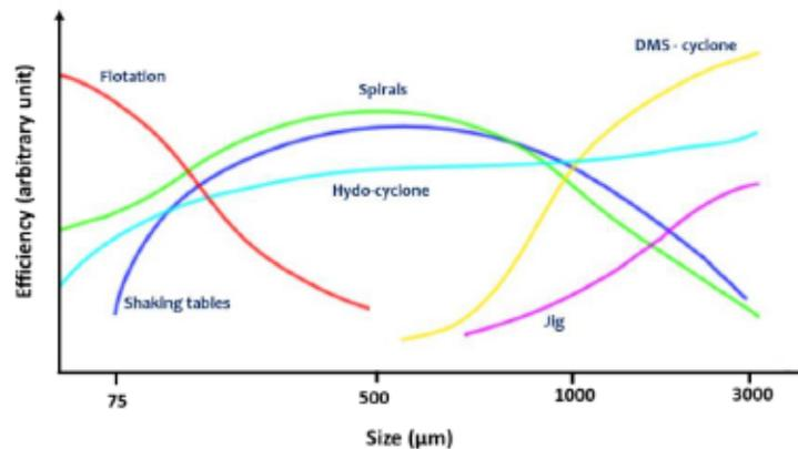
Figure 2.12 Comparison of some separation techniques efficiencies. Adapted from Hesford and Wellings, 1988
