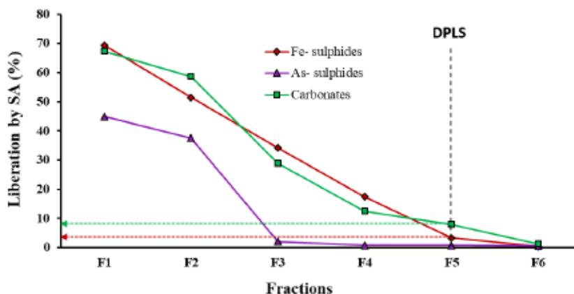
Figure 6.6 Free sulphide and free carbonate liberation degrees versus grain-size fractions.
