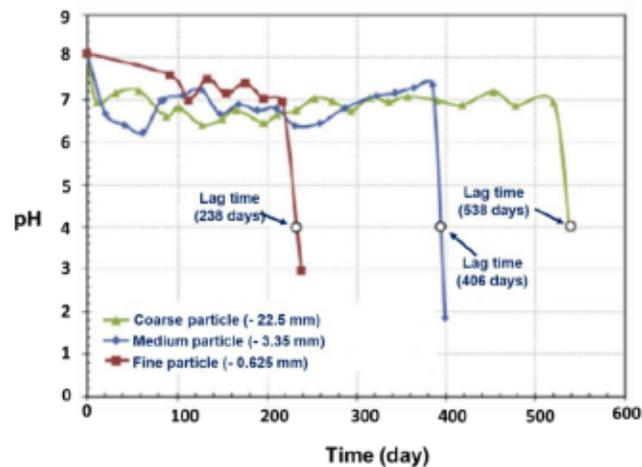
Figure 1S: Result of pH monitoring of a sample at different particle sizes. Adapted from Erguler and Erguler, (2015)
