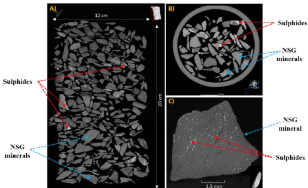
Figure 6.7 Mapping of sulphide minerals within the coarser specimen sample (WR > 5mm) using CT. Spatial distributions of sulphides in A) vertical and B) horizontal sections (X-slice) from the tomogram of the scanned specimen sample. C) Grain showing sulphide distribution at its surface. The light grey to white areas of the images represent sulphide minerals, and the grey areas are non-sulphide gangue (NSG).
