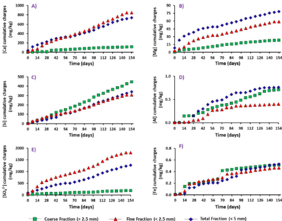
Figure 6.11 Calcium, magnesium, silicon, aluminum, sulphate, and iron load in the studied fractions.
