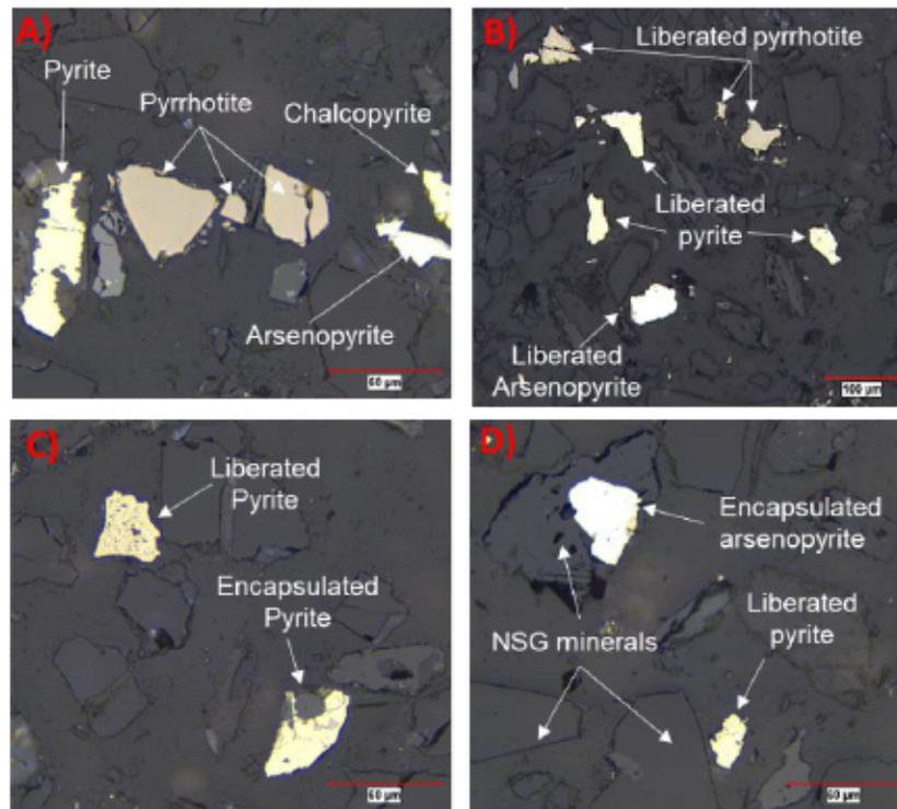
Fig. 6.3 Optical microscopy images illustrating sulphides and their liberation states: A) sulphide mineral observation, B) liberated sulphides, C) and D) sulphides partially liberated and/or totally encapsulated within NSG minerals.
