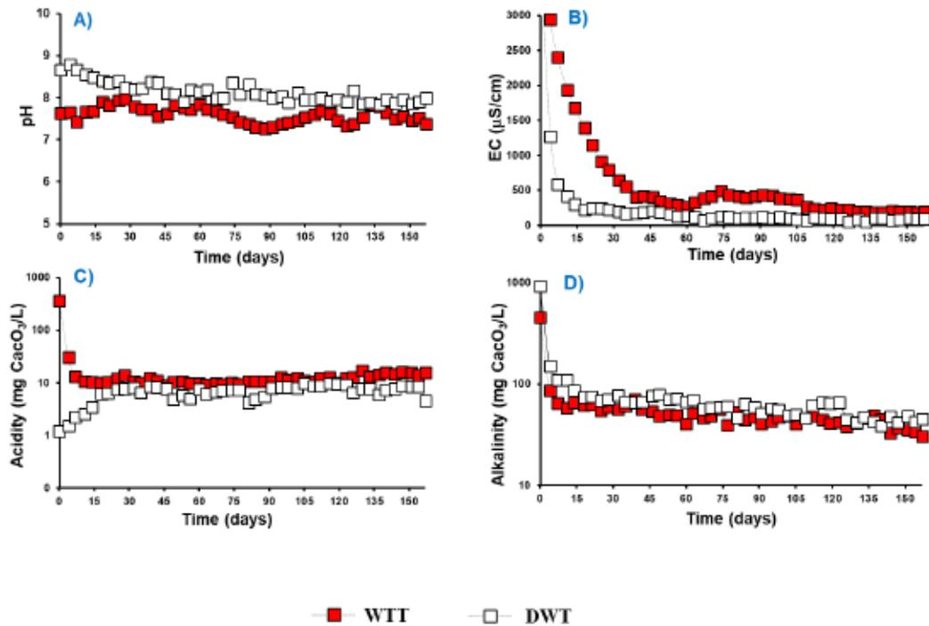
Figure 5.13 (A) pH, (B) electrical conductivity, (C) acidity, and (D) alkalinity evolution within the leachates from the WTT and DWT tailings.
