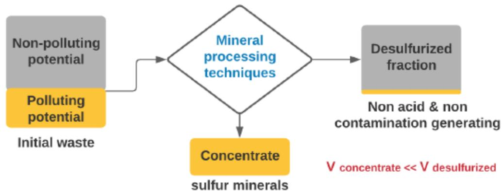
Figure 2.4 Principle of environmental desulfurization of mine wastes
