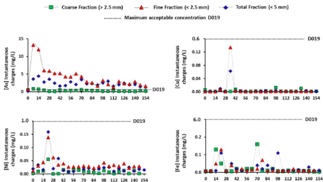
Figure 6.12 Instantaneous As, Cu, Ni, and Fe concentrations within the studied fractions (D019 corresponds to directive 019 which is environmental standard used in Quebec (Canada) for mining projects).
