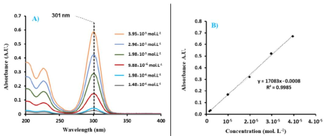
Figure 4.5 Absorbance of xanthate collector in UV–Vis A) as a function of wavelength ( $\lambda$ ) and B) as a function of collector concentration ( $\text{mol. L}^{-1}$ ) at 301 nm.
