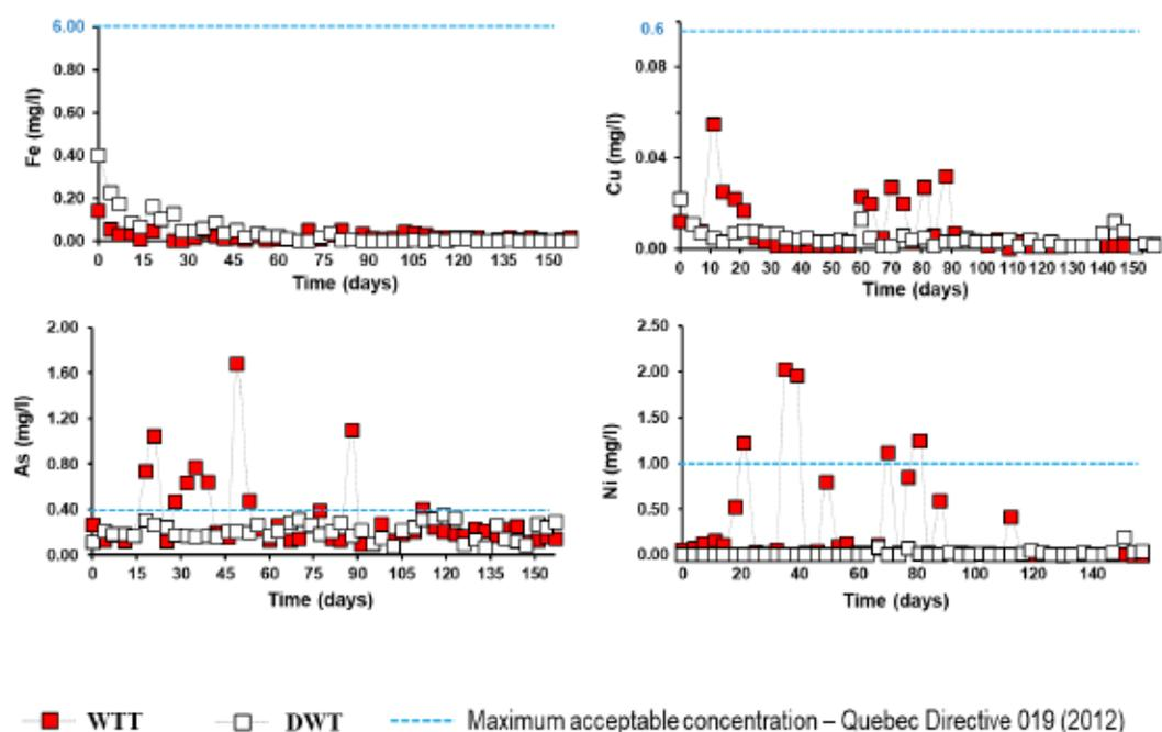
Figure 5.15 Contaminants (Fe, Cu, As, and Ni) leaching within WTT and DWT.
