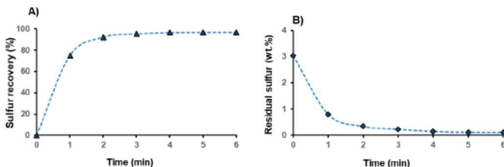
Fig. 5.9 Sulfur flotation kinetic of the Whale Tail tailings (desulfurization): A) Sulfur recovery vs. time; B) Residual sulfur vs. time.
