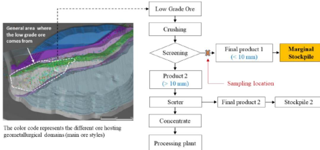
Figure 6.1 Sampling and simplified sorting plant concept.
