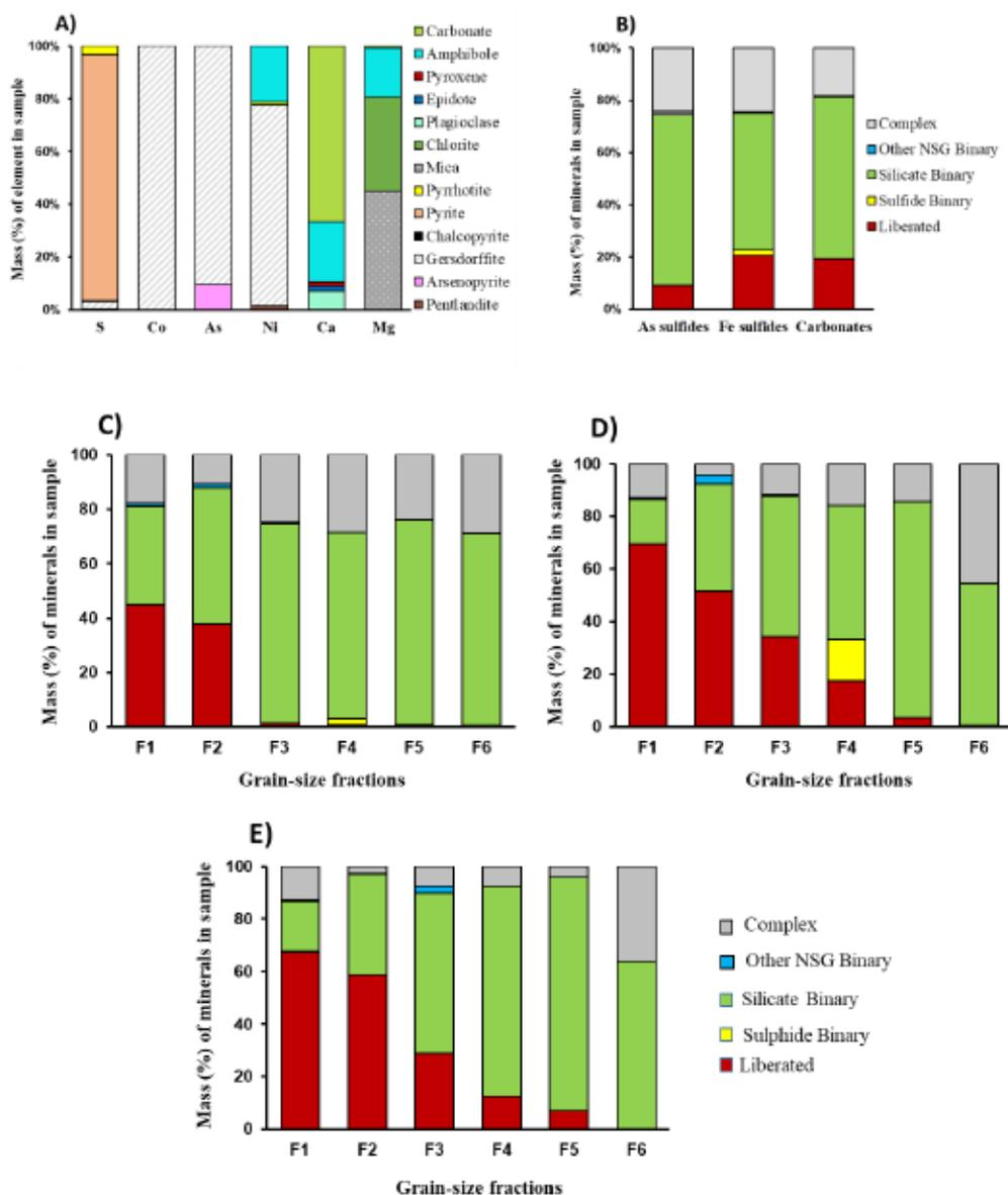
Figure 6.5 Element department and mineralogical associations of the studied WR and corresponding fractions: A) S, Co, As, Ni, Ca, and Mg department; B) mineralogical associations for carbonates and sulphides within the WR; and C) mineralogical
