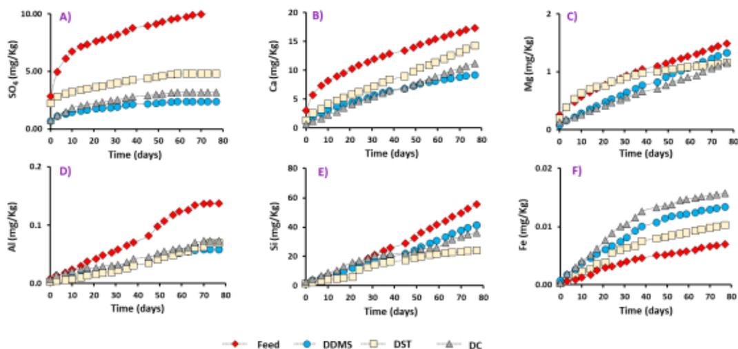
Figure 7.10 Evolution of the chemical quality of the leachates from the feed and desulphurized materials: A) SO<sub>4</sub><sup>2-</sup>, B) Ca, C) Mg, D) Al, E) Si, and F) Fe. Concentrations are presented as cumulative and mass normalized.
