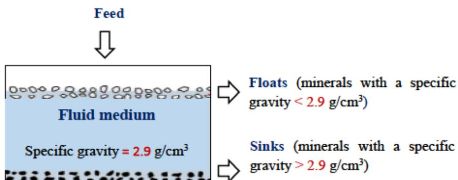
Figure 2S: Basic principle of DMS (specific gravity of fluid medium was 2.9 for illustration)
