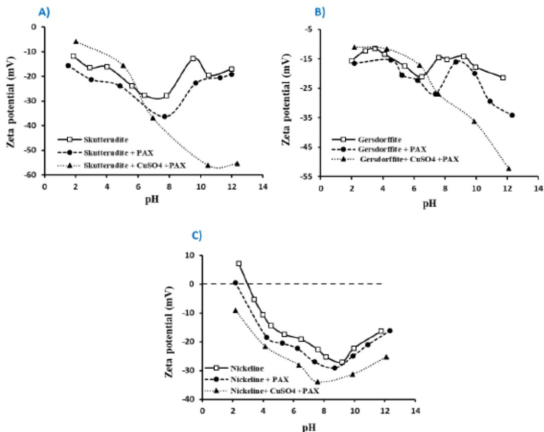
Figure 4.9 Zeta potential of A) skutterudite, B) gersdorffite, and C) nickeline as a function of pH in the presence/absence of the activator ( $10^{-3}$  mol/L  $\text{CuSO}_4$ ) and collector ( $10^{-4}$  mol/L PAX).
