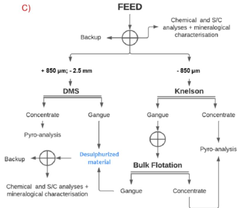
Figure 7.3 A process flow chart of the different decontamination techniques used: A) DMS approach, B) spiral/shaking table approach, and C) combination gravity and flotation approach (suite).
