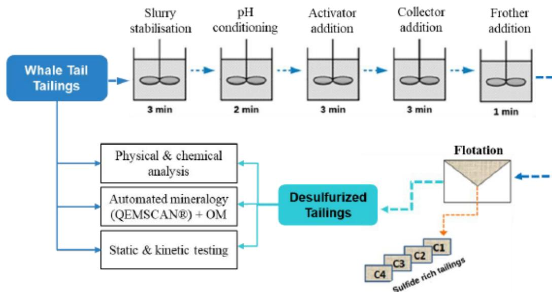
Figure 5.3 Flotation tests scheme.
