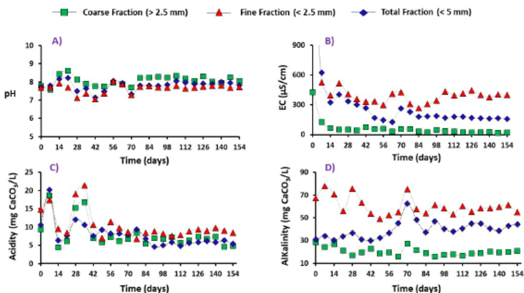
Figure 6.10 Evolution of pH, electrical conductivity, acidity, and alkalinity within the humidity cells.
