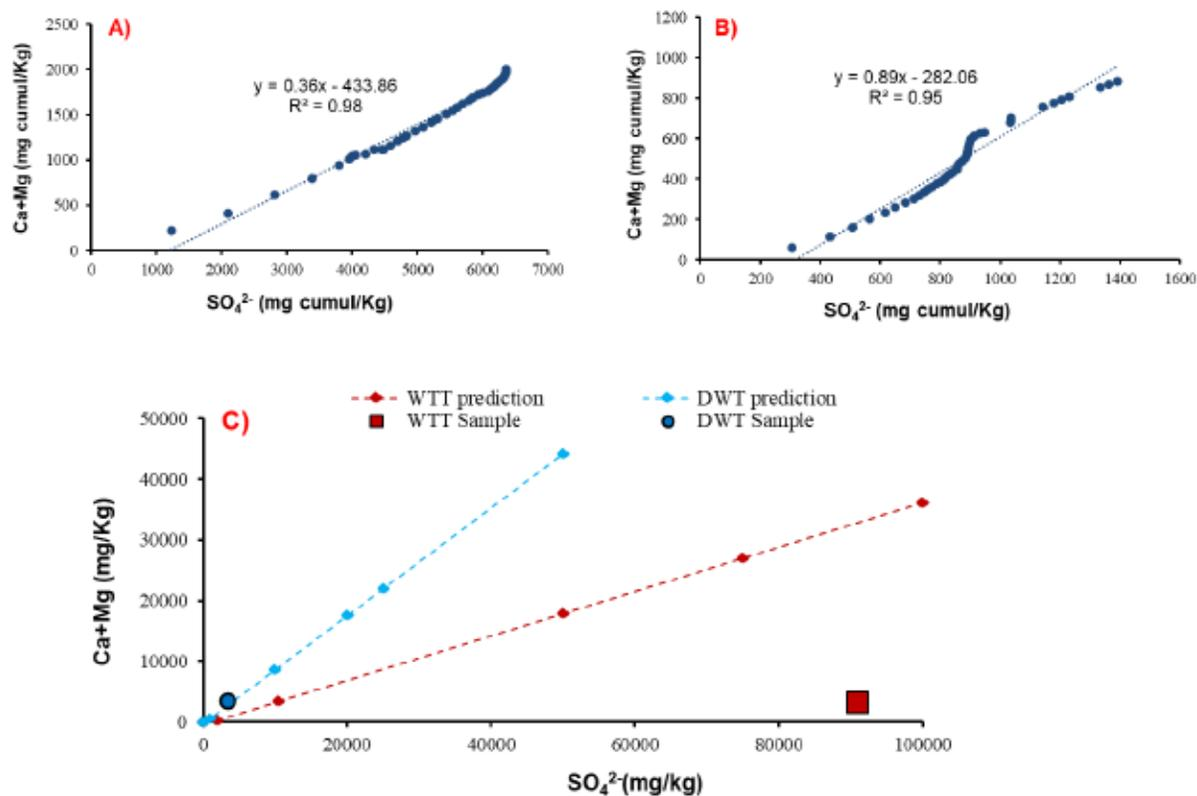
Figure S1.3 Long-term prediction of the geochemical behavior of WTT and DWT. A- B) Oxidation/neutralization predicted curves of WTT and DWT, and (C) experimental curves with projection of the initial composition of the samples.
