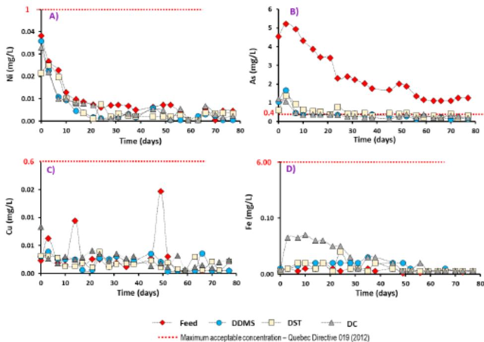
Figure 7.12 Contaminants (Fe, Cu, As, and Ni) leaching within the feed sample and desulphurized materials. A) Ni leaching, B) As leaching, C) Cu leaching, and D) Fe leaching.
