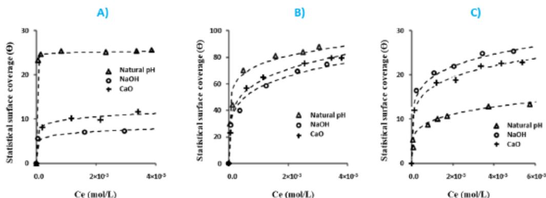
Figure 4.6 Xanthate adsorption isotherms on surfaces of A) skutterudite, B) gersdorffite, C) nickeline (under different pH value using NaOH and CaO regulator), and the corresponding Langmuir-Freundlich model fit.
