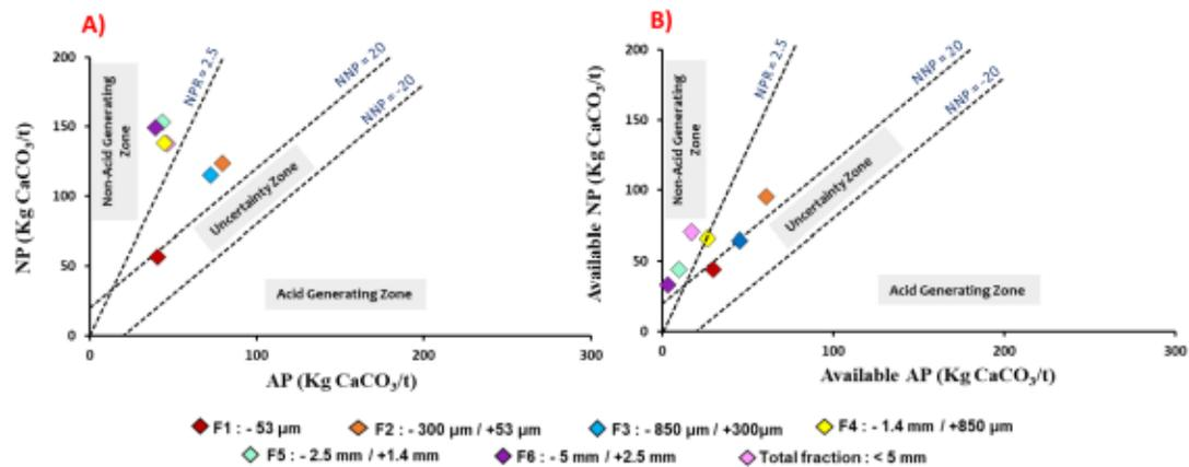
Figure 6.9 Graph illustrating results of acid generation potential through ABA tests with: A) absolute AP and NP, and B) available NP and AP (after correction with carbonate and sulphide liberation degrees).
