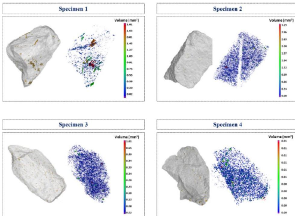
Figure 6.8 Volume distribution of sulphide minerals within some analyzed specimens.
