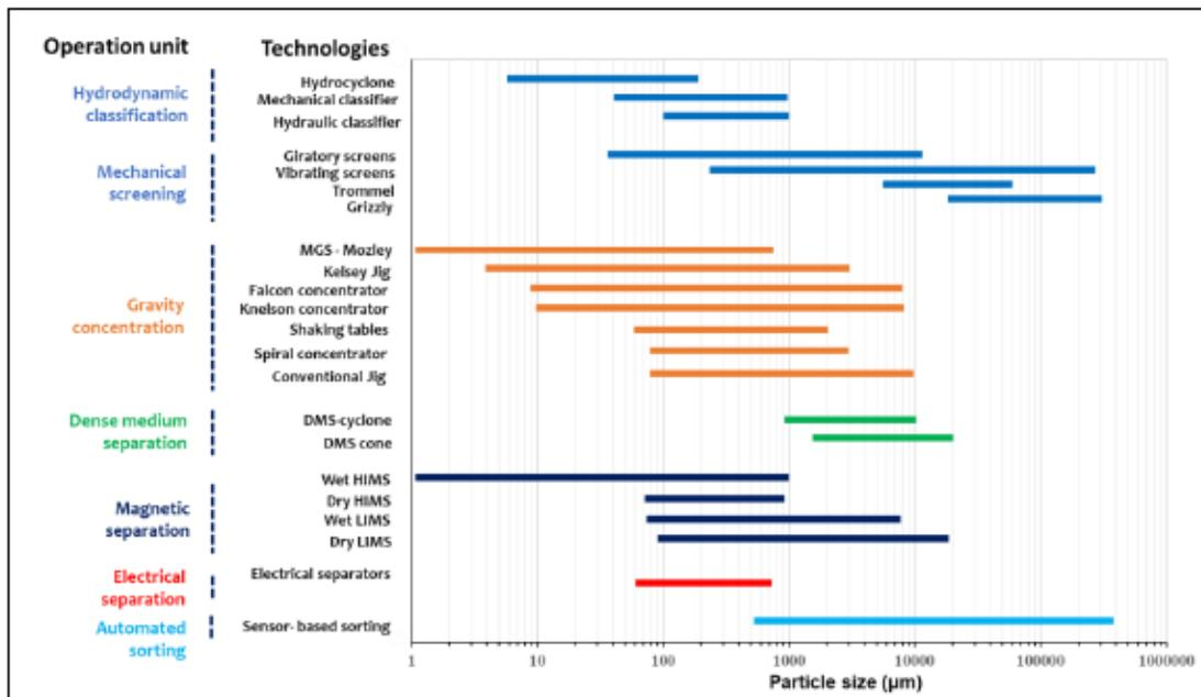
Figure 2.11 Suitable feed particle size ranges for the application of physical separation techniques. Adapted from Abols and Grady. (2006); Chatterjee. (1998); Dermont et al. (2008).
