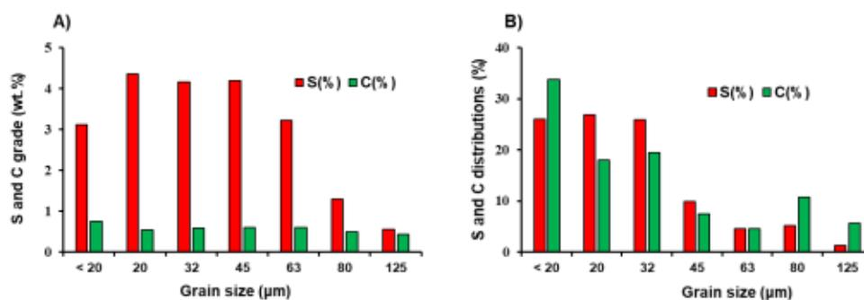
Figure S1.1 Size-by-size analyses of Whale Tail tailings. A) Grades of S and C in different grain size fractions. B) Distributions of S and C.
