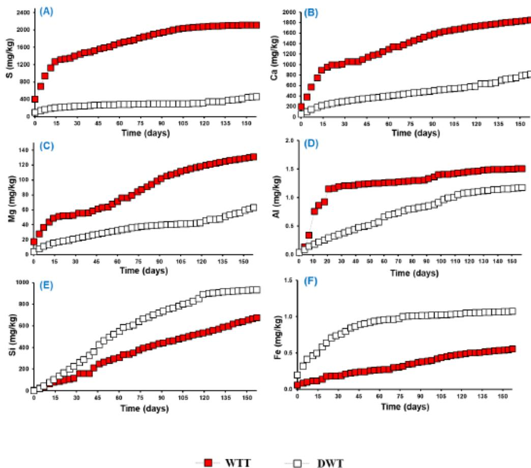
Figure 5.14 Evolution of the chemical quality of the leachates from WTT and DWT: (A) S, (B) Ca, (C) Mg, (D) Al, (E) Si, and (F) Fe. Concentrations are presented as cumulative, and mass normalized.
