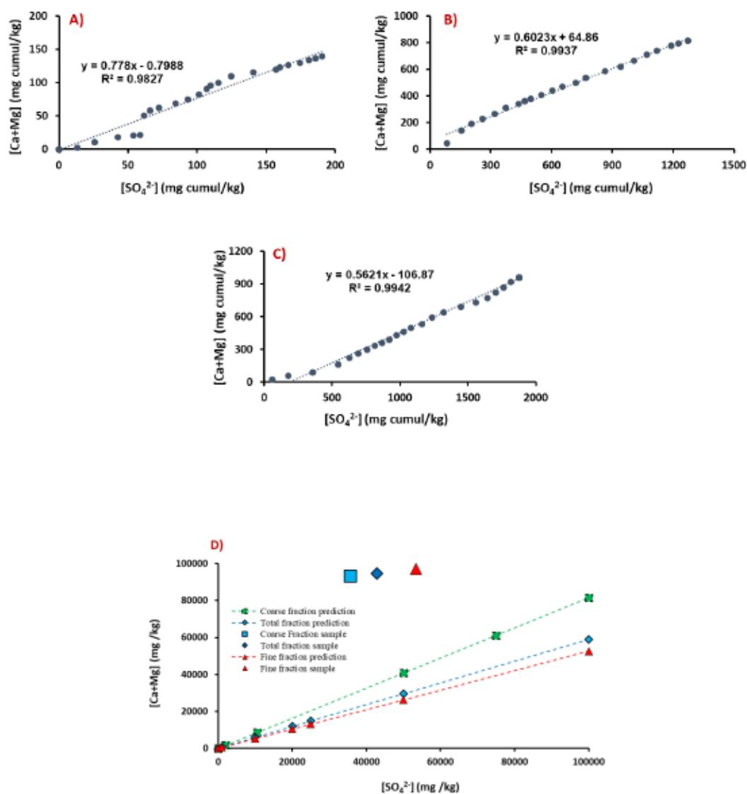
**Fig. S2.3** Oxidation/neutralization curves and long-term prediction of the coarse, total and fine fractions. A), B) and C): oxidation/neutralization experimental curves of coarse, total and fine fractions respectively and (D): long-term prediction for coarse, total and fine fractions
