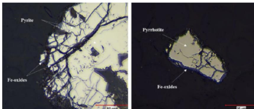
Figure 7.11 Optical microscopy images showing an example of pyrite and pyrrhotite coating with iron oxides.
