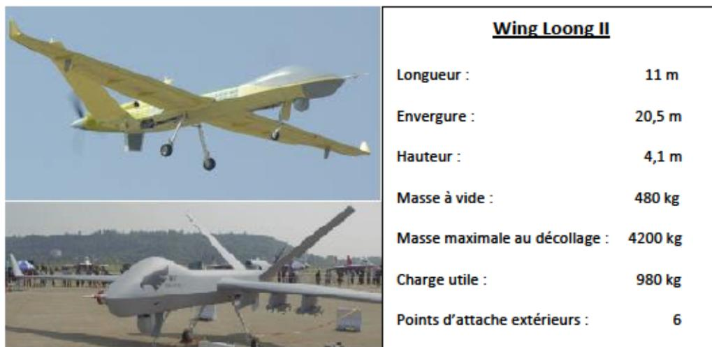
Figure 9 Drone de combat Wing Loong II.
