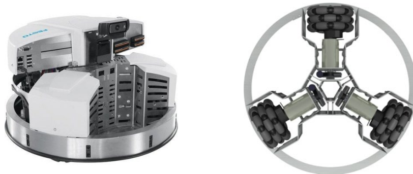
Figure 6 Robotino-Festo OMR and its Omni-drive
