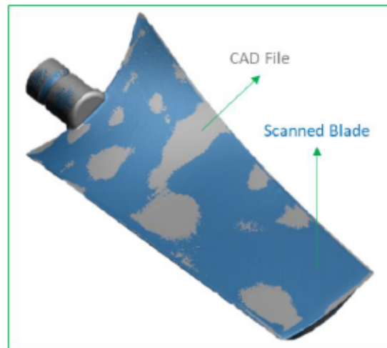
Figure 30 Comparison of the scanned blade with the 3D CAD file
