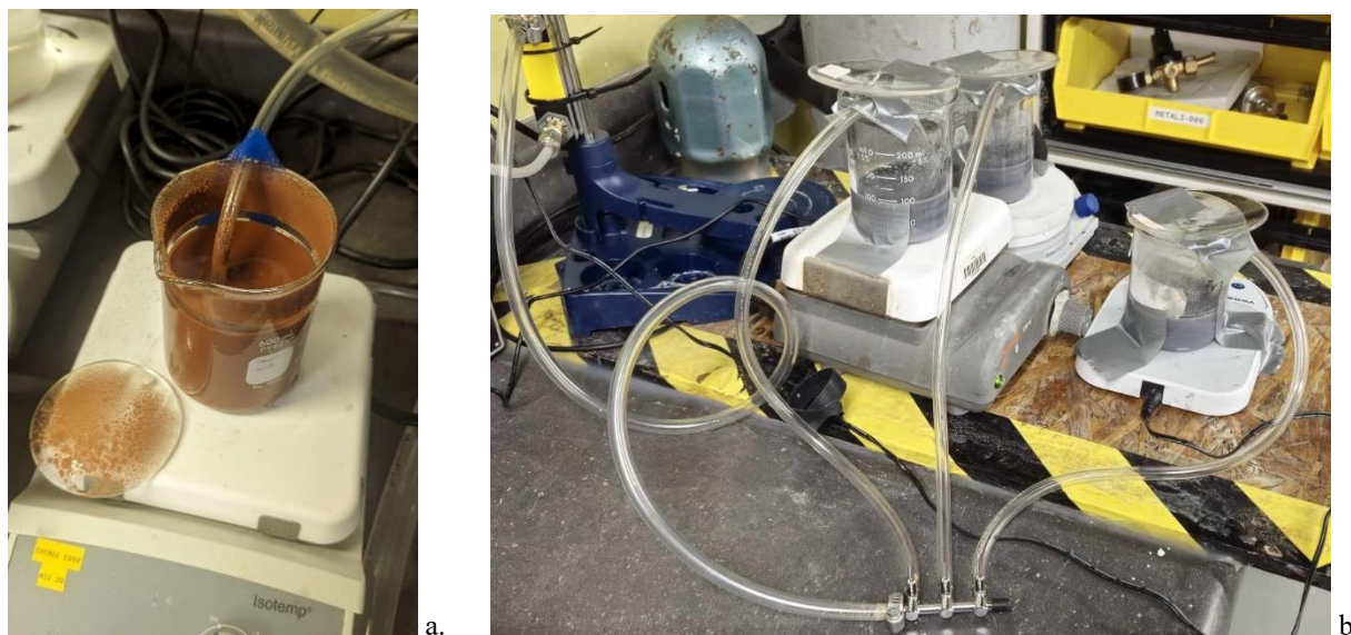
Figure 3-10 Set-up used for the \text{CO}_2 injection during the carbonation step for the experiments conducted one at a time (a) or in triplicates simultaneously (b)
