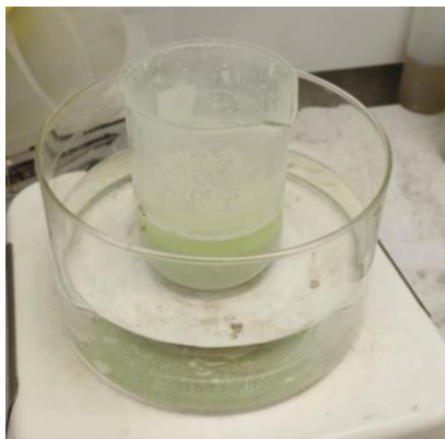
Figure 3-6 Neutralization-precipitation arrangement used to cool down the solution
