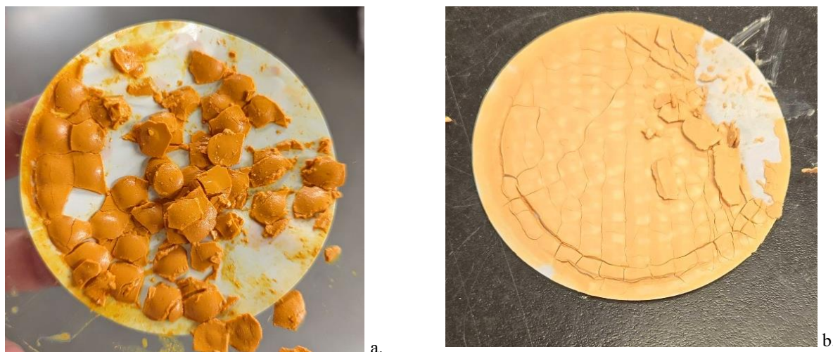
Figure 3-9 Changes observed in the coloration of co-precipitated REOHs before (a.) and after (b.) drying
