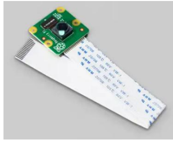
Figure 37 Camera Module standard[105]
