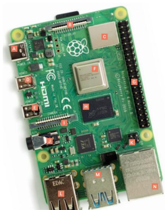
Figure 36 Les composants Raspberry Pi 4 type B[104]
