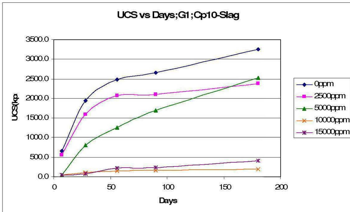
Figure 16: UCS vs Days for 72% fine particles; CP10: Slag
