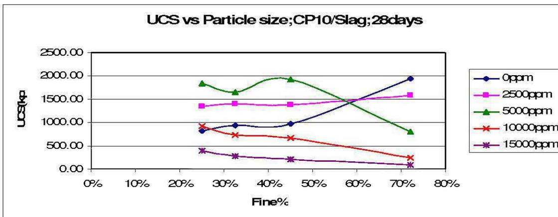
Figure 31: UCS vs Particle size; CP10: Slag; 28 days
