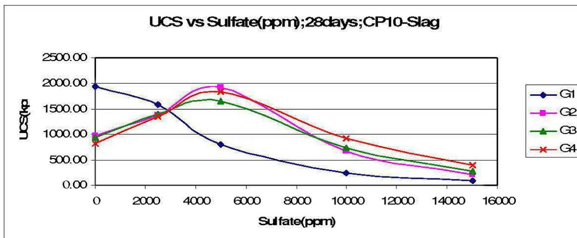
Figure 41: UCS vs Sulfate content; CP10: Slag; 28 days
