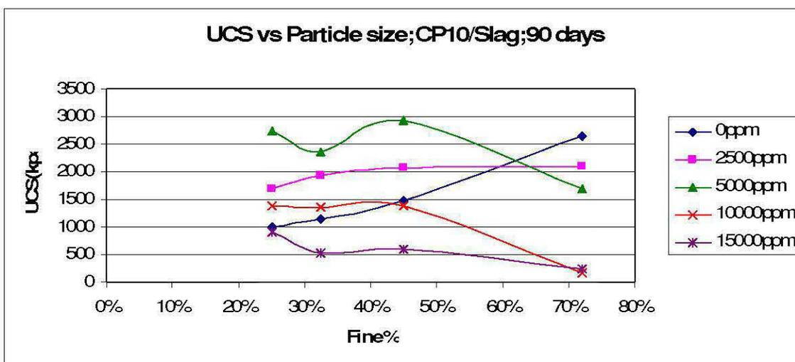
Figure 33: UCS vs Particle size; CP10: Slag; 90 days
