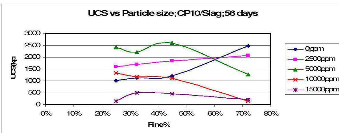
Figure 32: UCS vs Particle size; CP10: Slag; 56 days
