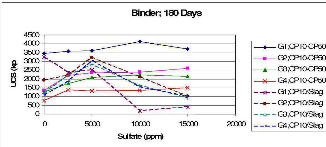
Figure 24: UCS according to the content sulfates for the CP10-CP50 and CP10-Slag (180 days of cure)
