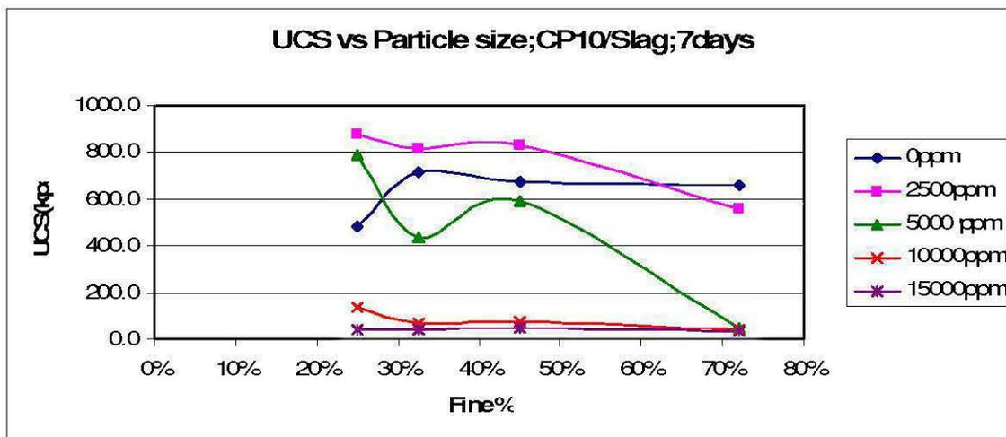
Figure 30: UCS vs Particle size; CP10: Slag; 7 days
