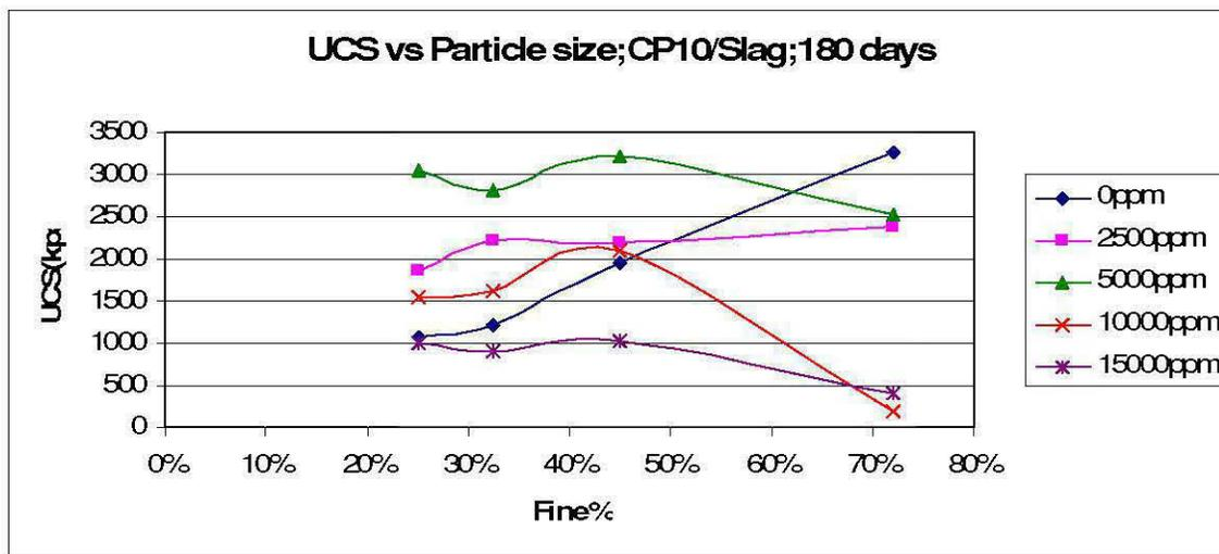
Figure 34: UCS vs Particle size; CP10: Slag; 180 days
