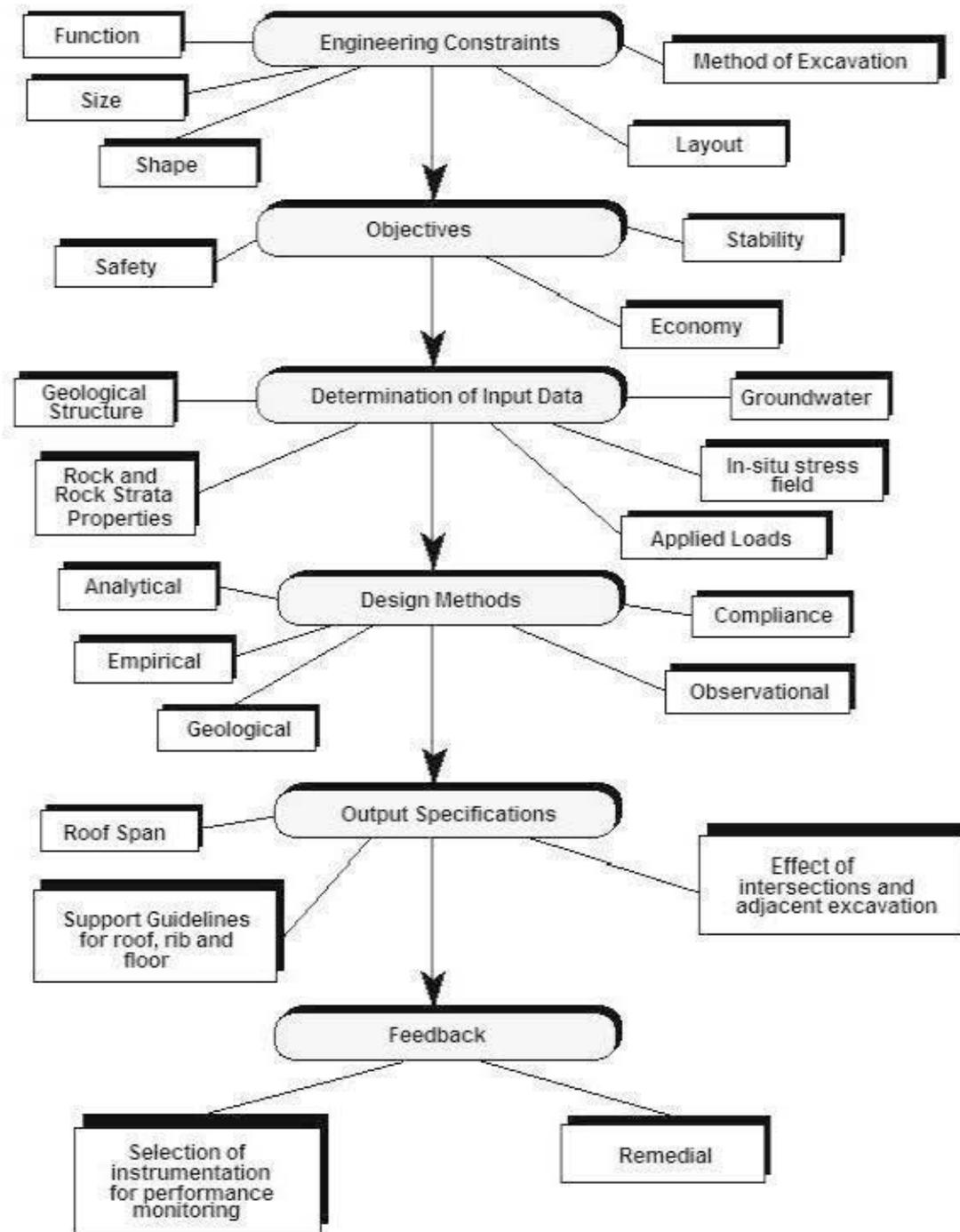
Figure 3: The flow chart showing a simplified design chart for underground mine design
