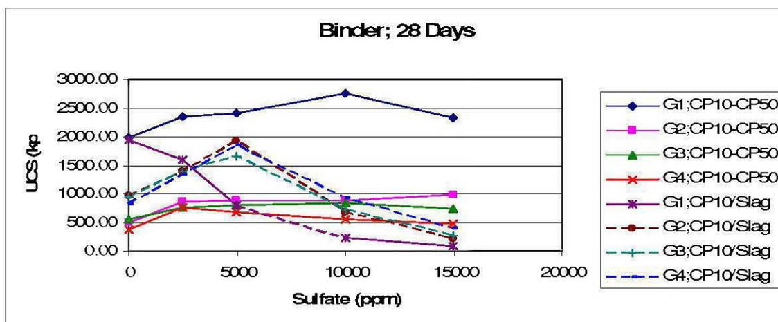
Figure 21: UCS according to the content sulfates for the CP10-CP50 and CP10-Slag (28 days of cure)
