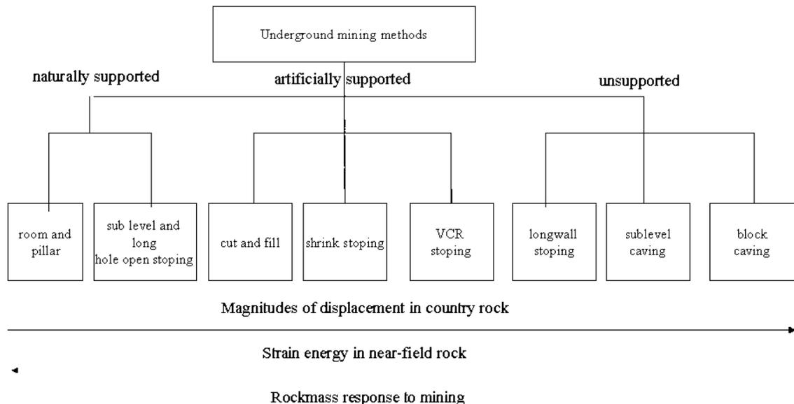
Figure1: Diagram showing a breakdown of mining methods according to the mine regional support system used, Brady and Brown (2004)
