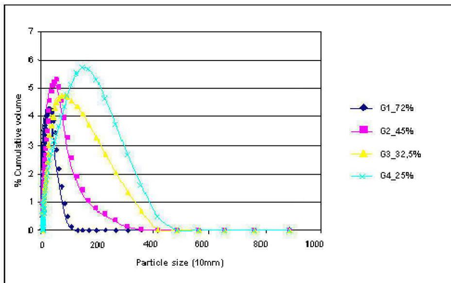
Figure 8: Histogram of Particle size distributions of the silica powder
