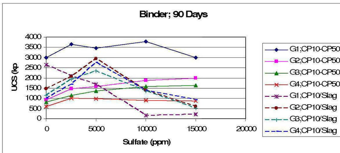
Figure 23: UCS according to the content sulfates for the CP10-CP50 and CP10-Slag (56 days of cure)
