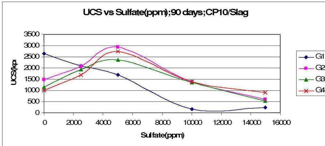
Figure 43: UCS vs Sulfate content; CP10: Slag; 90 days
