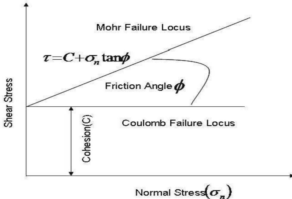
Figure 2: Mohr Failure Locus
