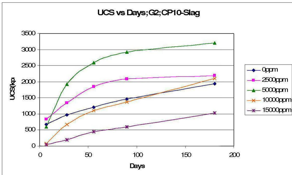
Figure 17: UCS vs Days for 45% fine particles; CP10: Slag
