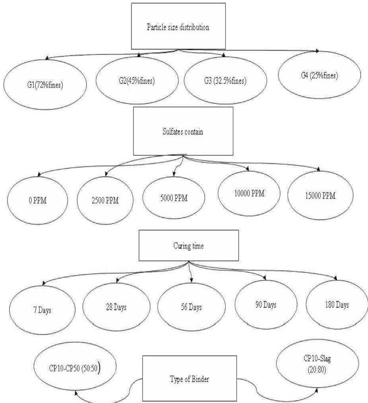
Figure 9: Chemical and physical factors which were considered to prepare laboratory samples
