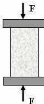
Figure 10: Simplified diagram of unconfined compression test to obtain UCS value
