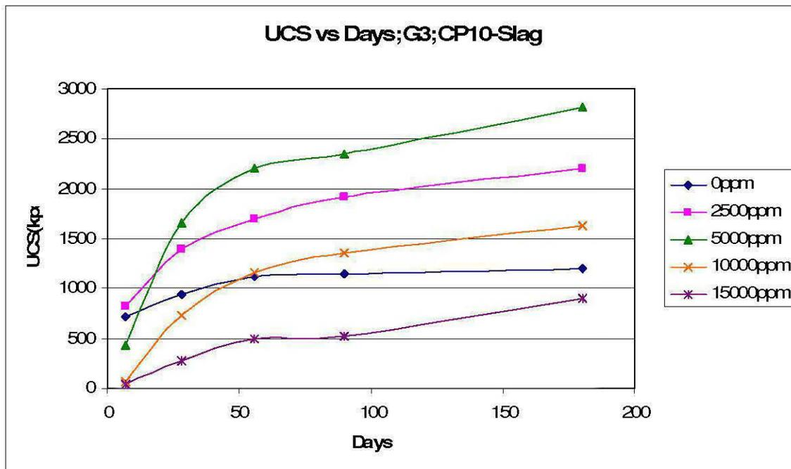
Figure 18: UCS vs Days for 32% fine particles; CP10: Slag
