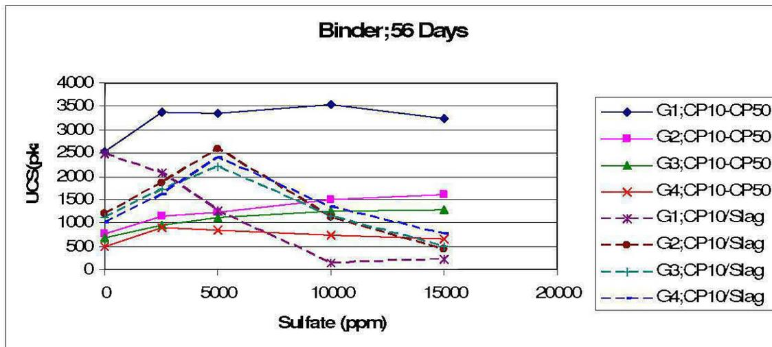
Figure 22: UCS according to the content sulfates for the CP10-CP50 and CP10-Slag (56 days of cure)
