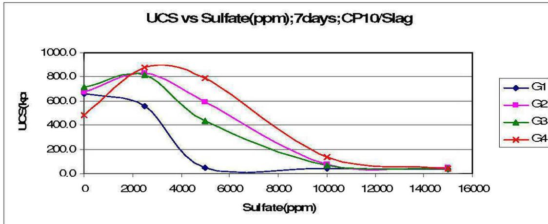
Figure 40: UCS vs Sulfate content; CP10: Slag; 7 days
