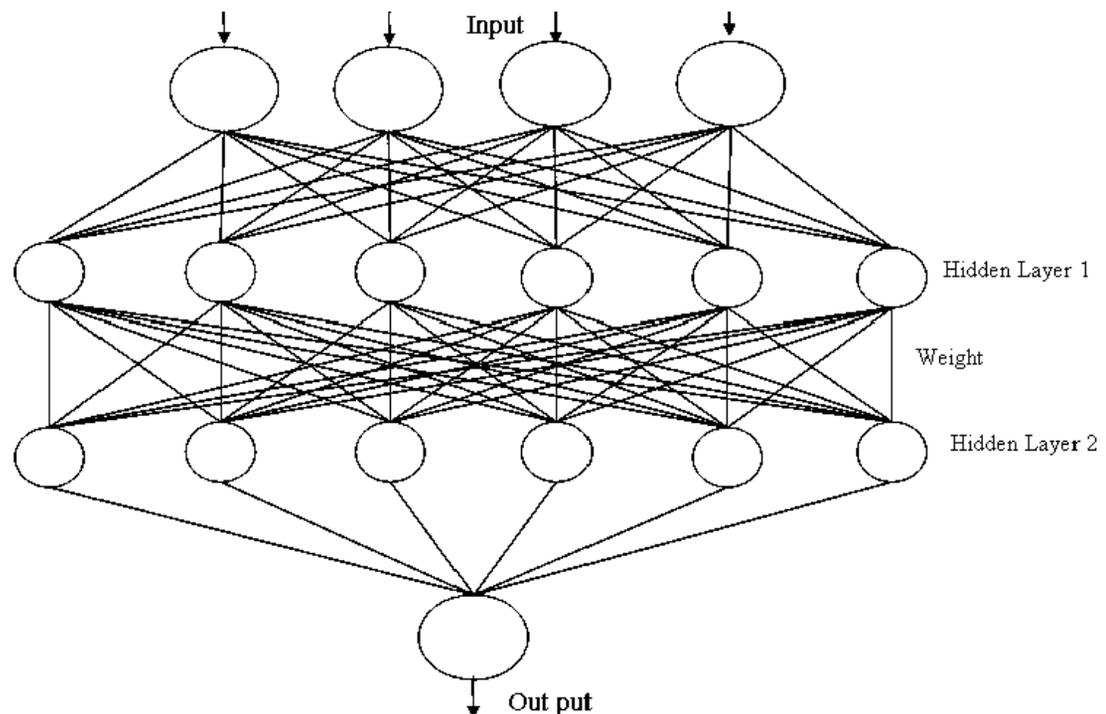
Figure 5: Structure of multi-layered type artificial neural network
