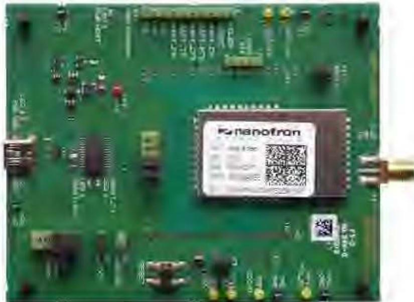
**Figure 4.63:** Nanotron Sensor. [46]
