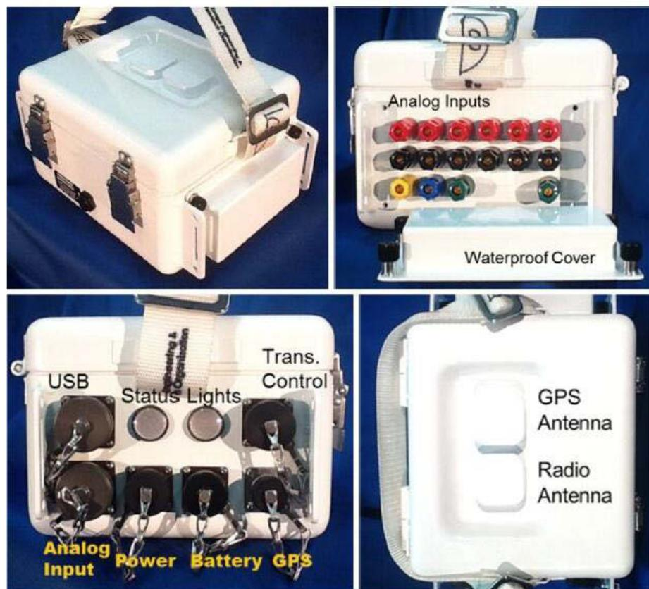
Figure 3.3 The Zonge Electromagnetic Network (ZEN) receiver (Source: Zonge International Inc.).
