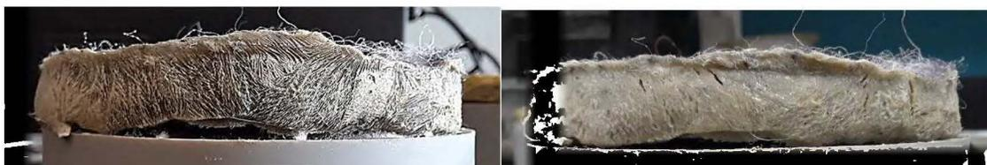
Figure 4-5 : Cracks in GCL specimens permeated with DIW – under free-swell permeation conditions (details in Chev e, 2019). a) Frozen at  $\approx 5 \text{ }^\circ\text{C}$ . b) Thawed at the ambient temperature of  $\approx 21 \text{ }^\circ\text{C}$ .
