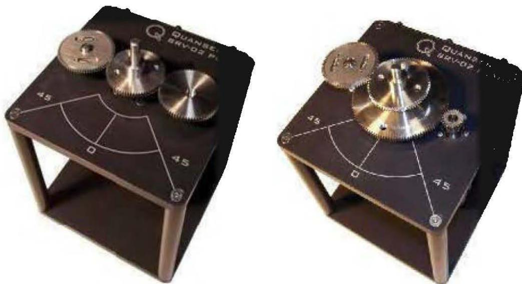
(a) Configuration "Low-Gear Ratio"
